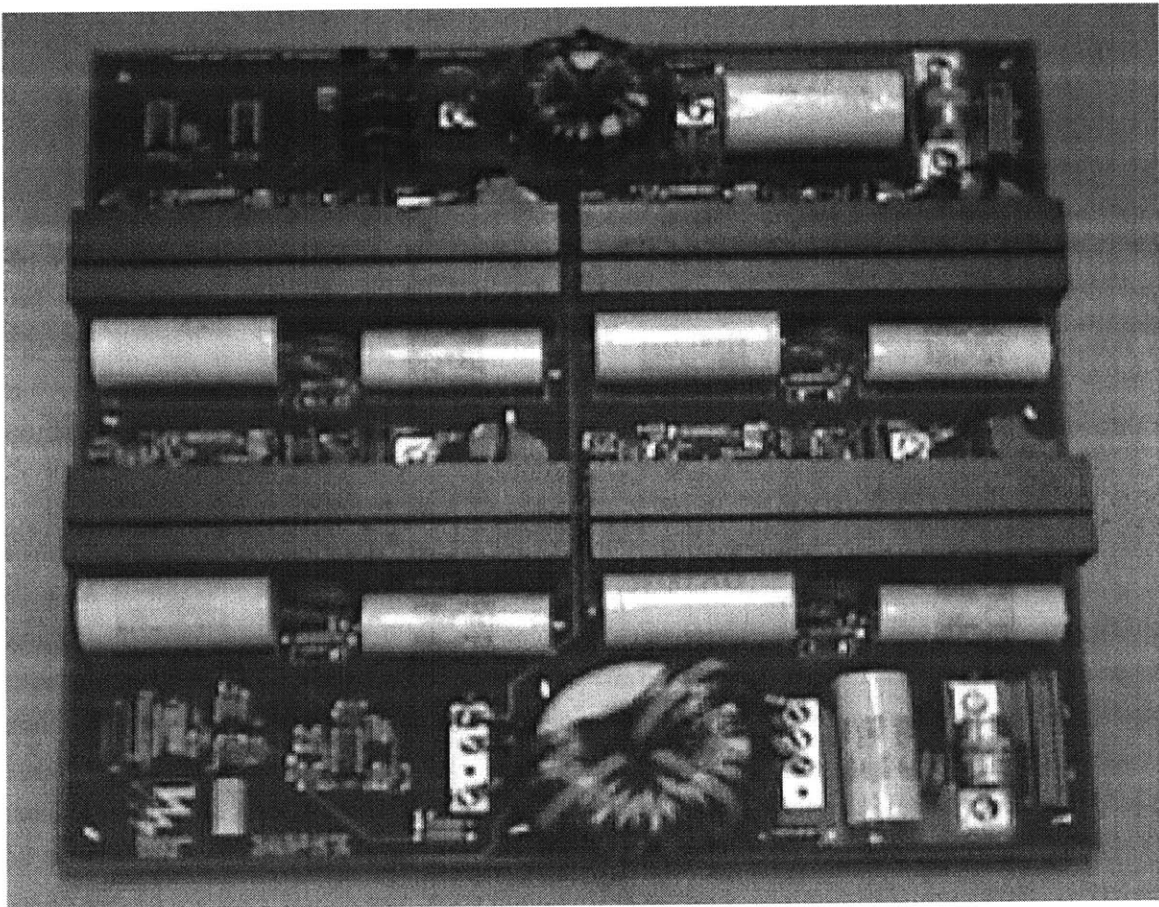
Figure 6.19: Experimental prototype of the four cell interleaved buck converter using average current-mode control. The electronics for the cells are primarily located near heat sinks on which the power MOSFET and diode for each stage are mounted. The wound coils at the top and bottom are a part of the input and output EMI filters, respectively.
