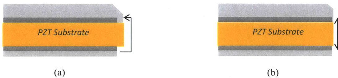
Figure 5-1: Reduction of distance between metal sides after sanding edges; (a) initial space between metal sides; (b) effect of removal of PZT material and the reduction in space between metal sides.
