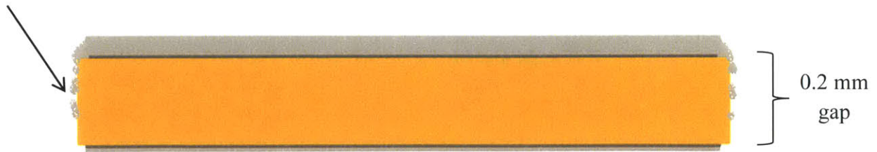
Figure 3-6: Nickel overspray during sputtering that might lead to arcing.
