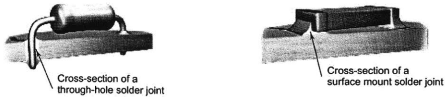
Figure 3-4: The two main methods of securing electronic components to PCBs differ in regards to the location of their leads (a) through-hole technology solders leads through the PCB (b) surface mount technology solders leads on top of the PCB. [21]
