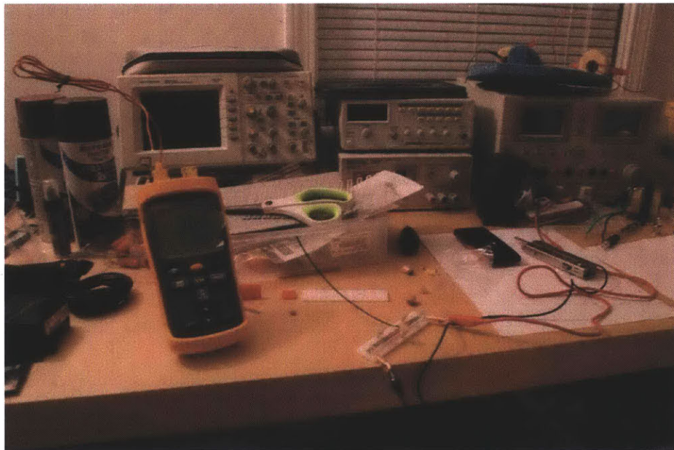
Figure 5-6: Preliminary desktop experimental setup with 15V 3A power supply, hand-held thermocouple thermometer, and PMMA bonding jig
