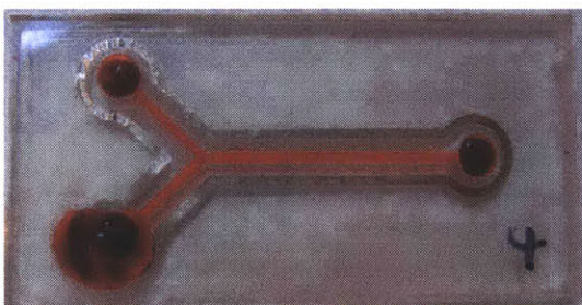
(e) Knauf's closed loop, 1mm thick, etched 7.5μm thick Ni susceptor following channels at heating from Fluxeon an offset of 1mm come close to a complete seal
