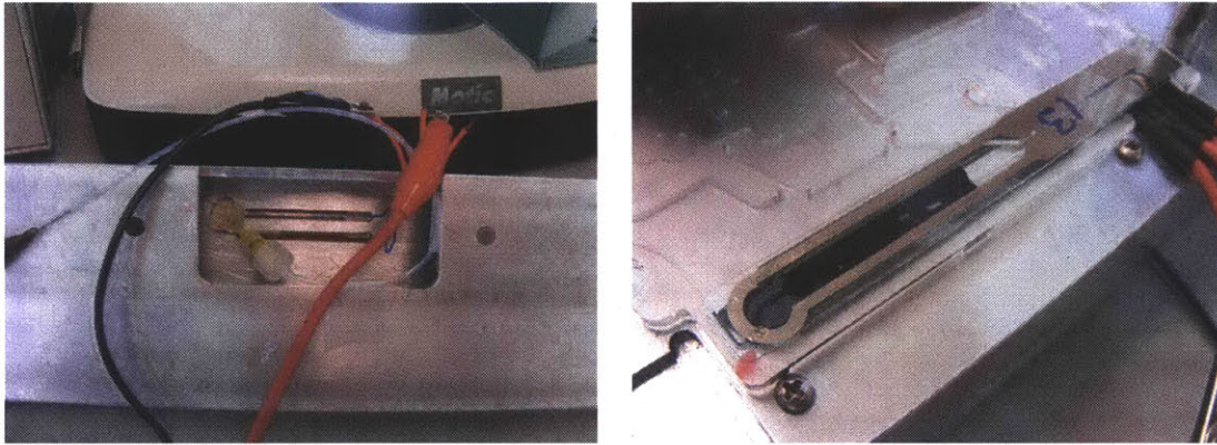
(a) Two sided cuvette bonding and ink test (b) Ink fills cuvette without overflow within trace boundary
