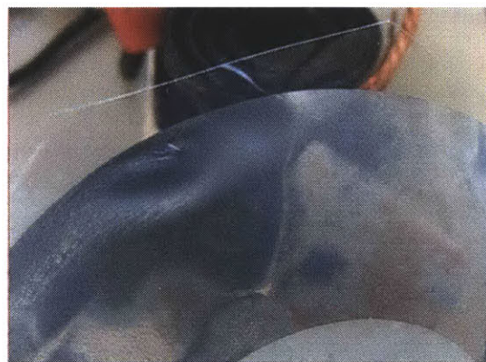
(d) Pancake coil melts PMMA with a large section of thin susceptor
