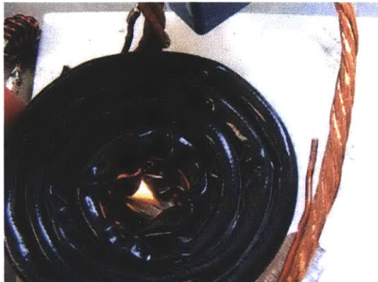
(c) Coil quickly heats kitchen foil to glowing temperatures
