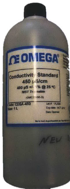
Figure 4-8: Omega conductivity solution used to prepare solution standards for electrode calibration.
