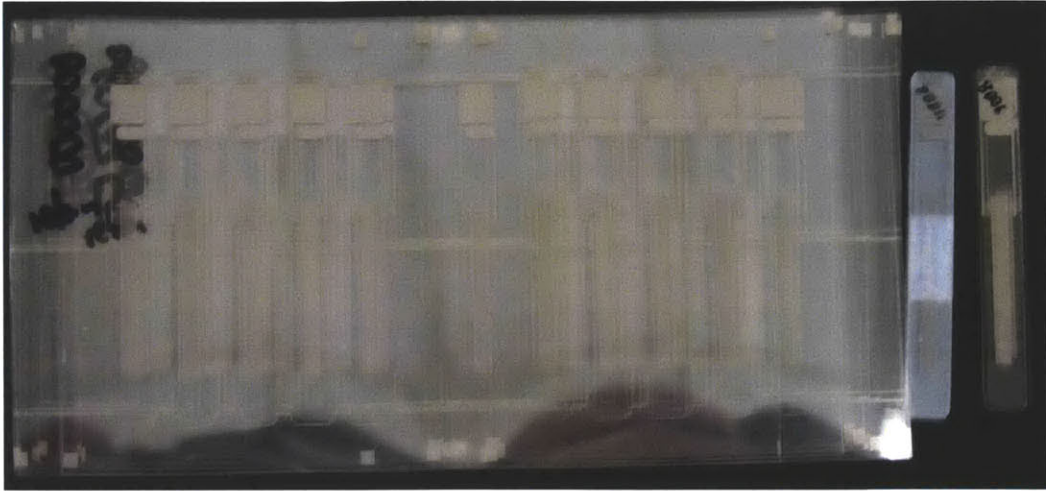
Figure 4-6: Series of electrodes before die cutting on left, single cut electrodes on right.
