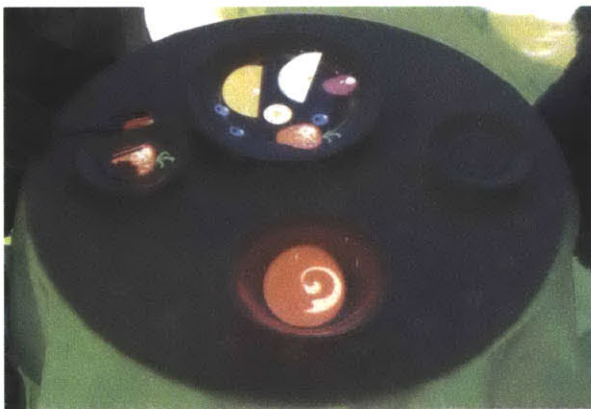
Figure 6: Play table with physical plates, trackable fork, and projected digital fruit and chocolate dip.
