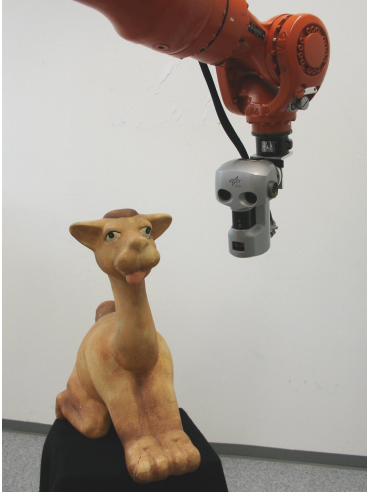
(a) A camera and laser-equipped 3D modeling sensor mounted on a robotic manipulator.
