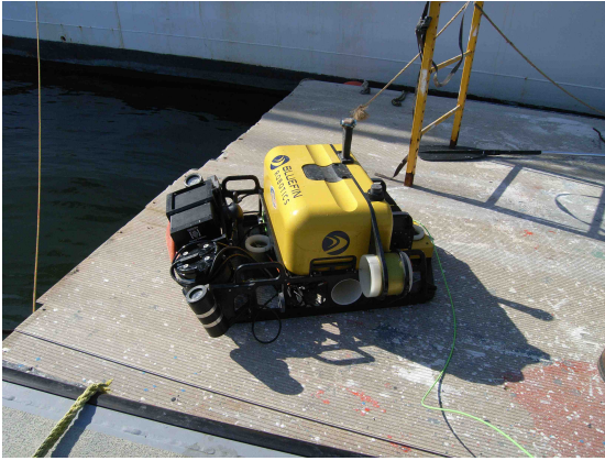
(a) The HAUV, version HULS3, prior to deployment at the stern of the Seneca .
