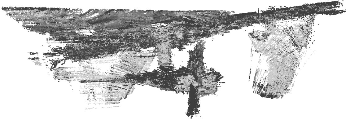
Figure 6-9: Composite point cloud showing the data collected from the planned inspection of the USCGC Seneca outboard stern. The alignment of each point's outward-facing normal vector with the camera viewpoint depicted in this image is reflected by the shading of each point. Points with normals directed toward the camera are light gray in color, and points with normals directed away from the camera are dark gray in color.
