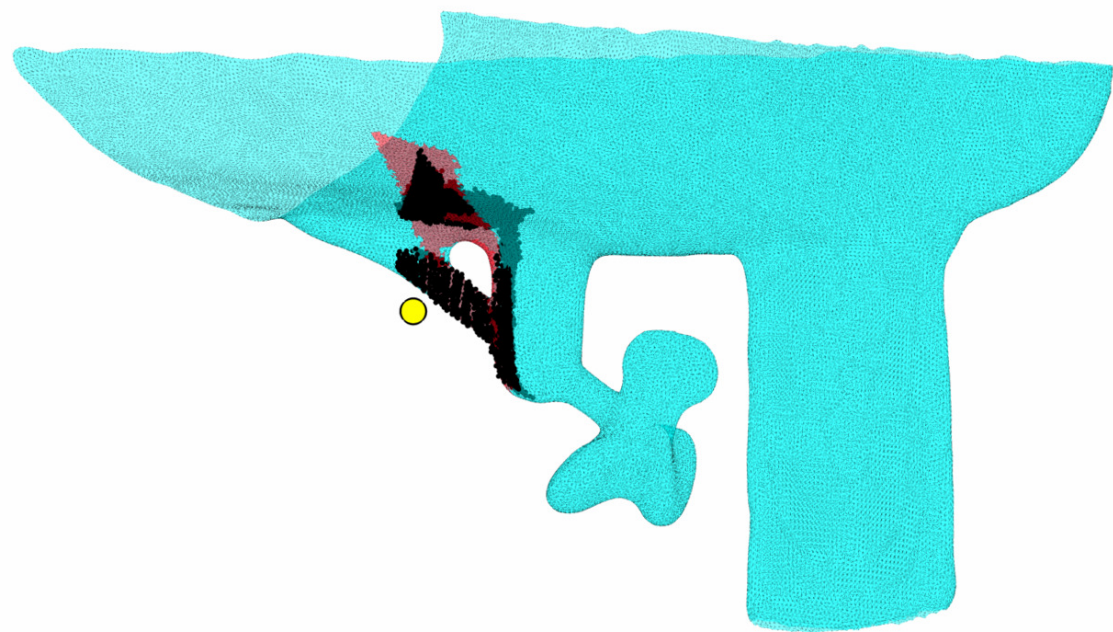
(b) View of shaft, showing a larger gap between shaft and hull than modeled.
