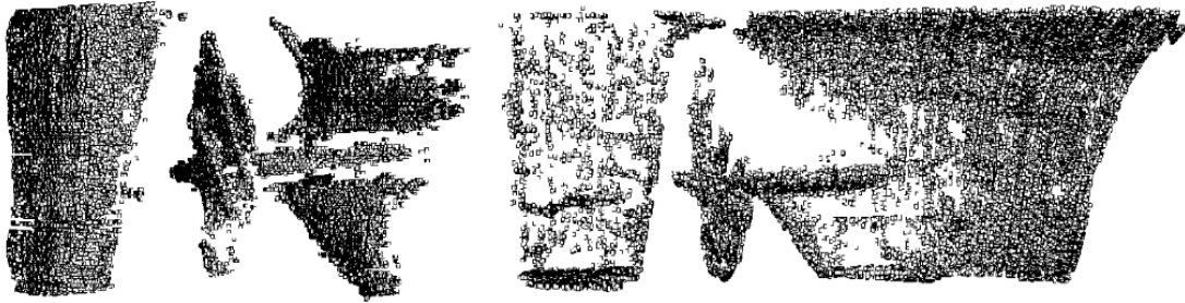
(a) Raw-data point clouds obtained from the starboard-side wall and bottom wall of the identification survey, respectively.
