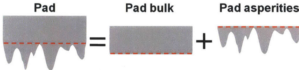
Figure 2.16: Pad structure assumption in physical die-level CMP model. The whole pad is comprised of bulk and asperities.
