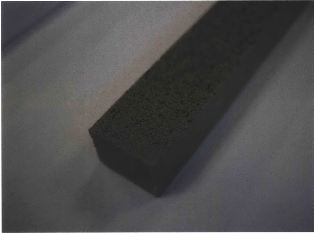
Plate 3 First columnar specimen cut open; higher density material is apparent at the lower bound of the cast.
