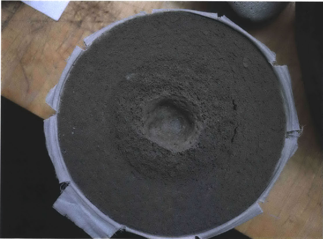
Plate 25 Centrifuged specimen prior to fabric sleeve removal
