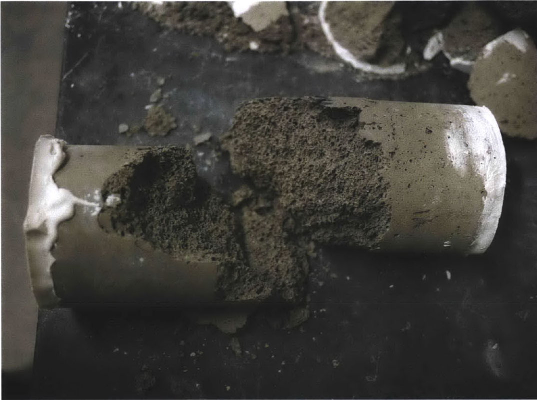
Plate 53 Aerated compression cylinder after testing (Specimen A1). Representative diagonal fracture pattern typical of brittle cellular solids is apparent.
