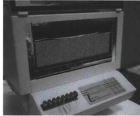
Figure 5.5.4 Steady state thermal testing setup using a LaserComp FOX 305 heat flow meter at the Fraunhofer Center for Sustainable Energy Systems, Cambridge, MA.
