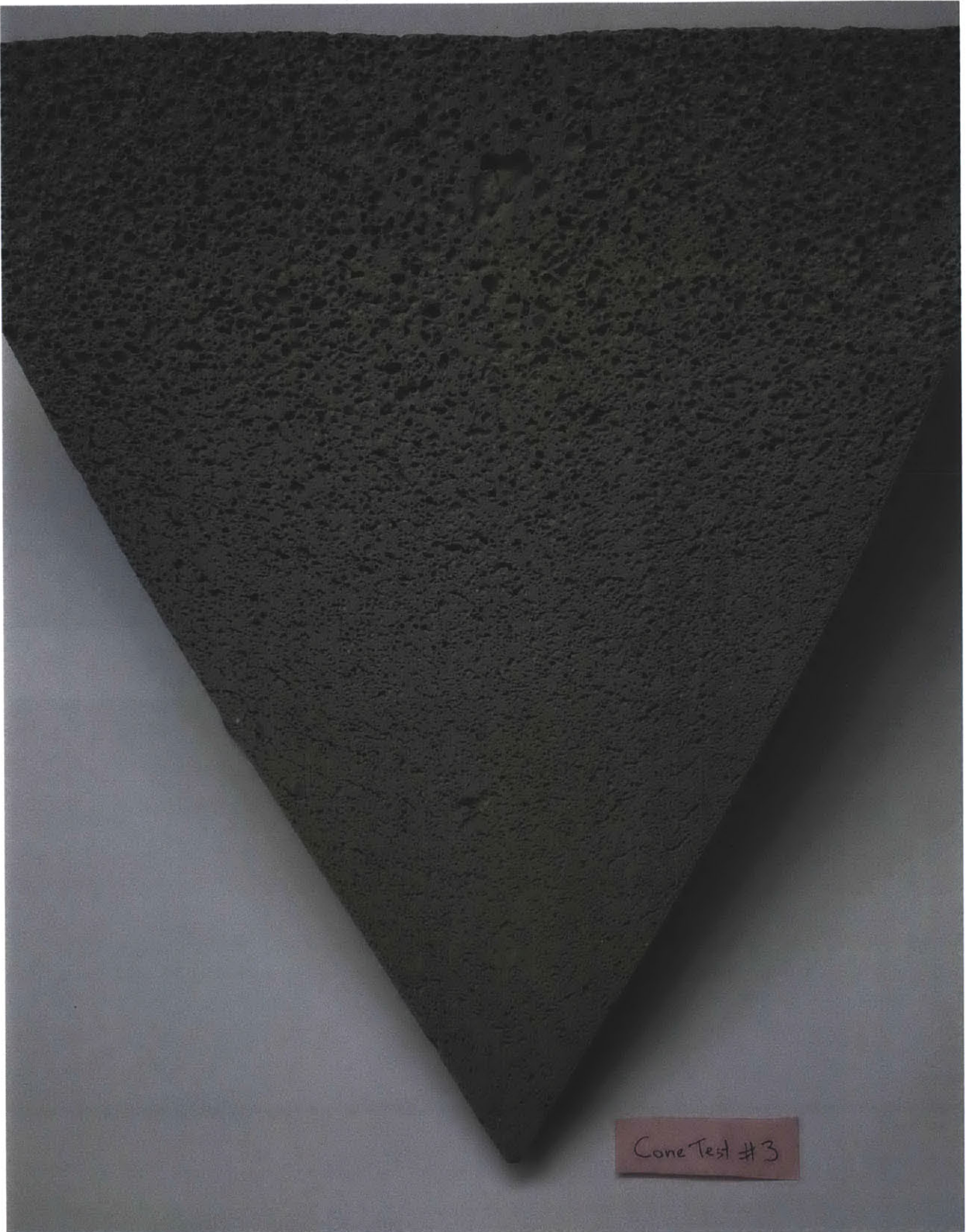
Plate 21 Internal cellular composition of fabric-formed conical specimen #3
