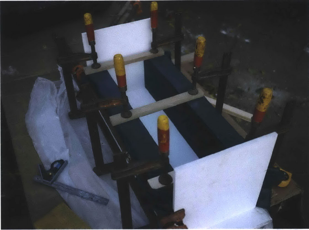
Plate 50 Second beam prototype molding setup. Blocks of gypsum on the sides of the mold are wrapped with fabric.
