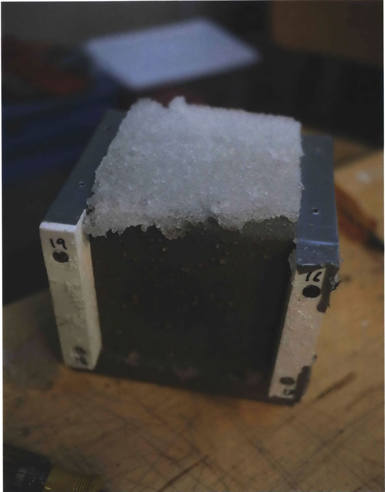
Plate 37 Partially demolded aerated concrete specimen cast in super absorbent polymers
