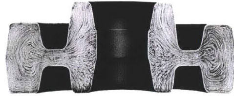
Figure 2.1.1 Flow structure of a hot-formed (forged) transmission gear blank. (DeGarmo 2003, 374)
