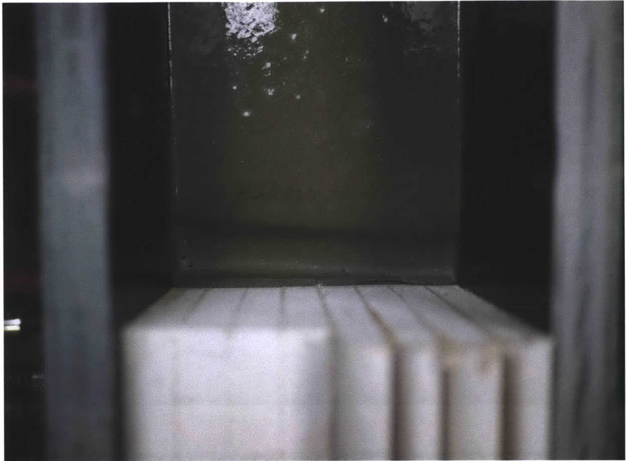
Plate 40 Retarded expansion visible at interface between gypsum and aerating slurry
