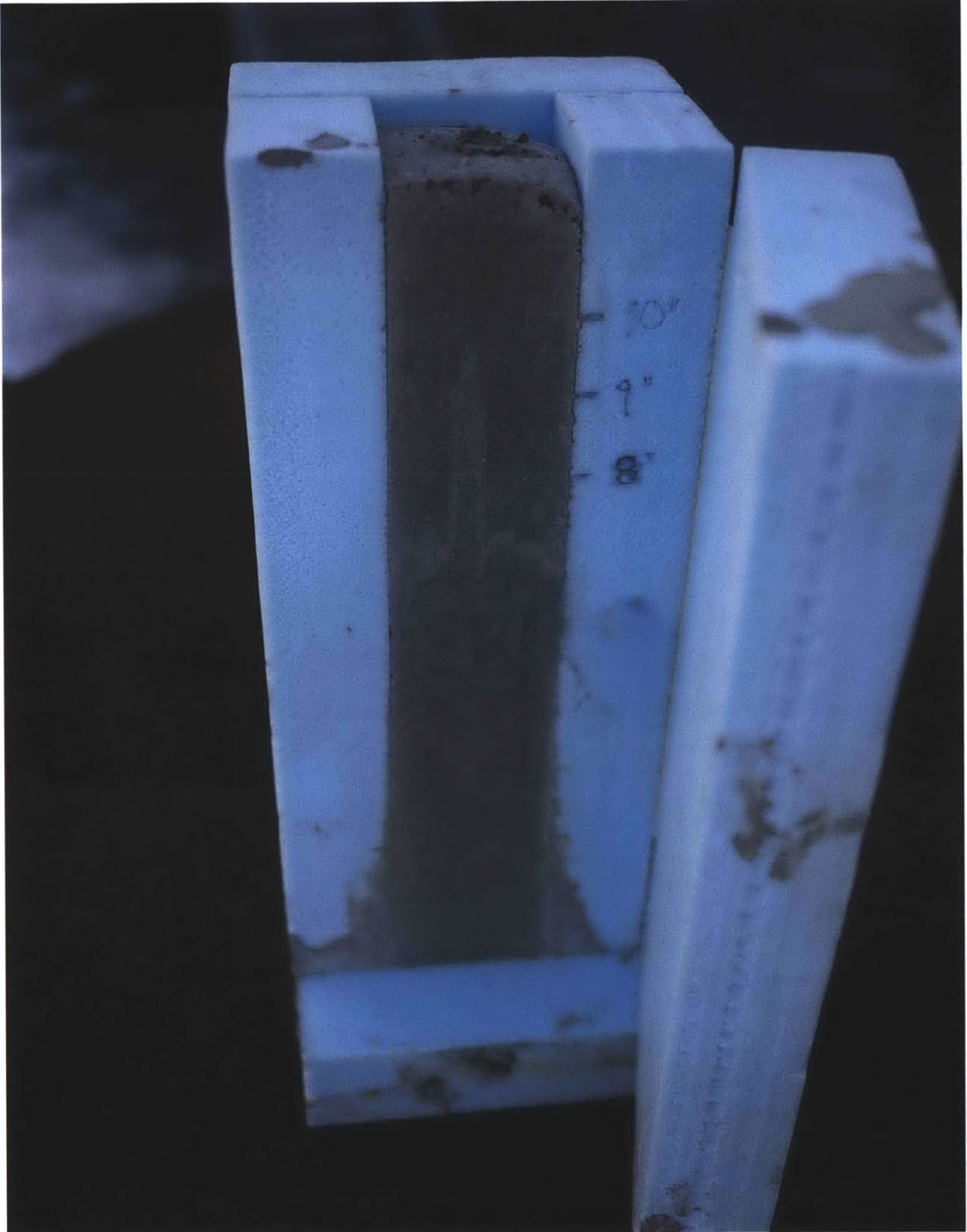
Plate 2 First gravity test column partially demolded
