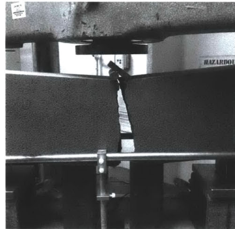
Figure 5.5.3 Beam prototype after 3-point bending test. Brittle fracture failure mode apparent.
