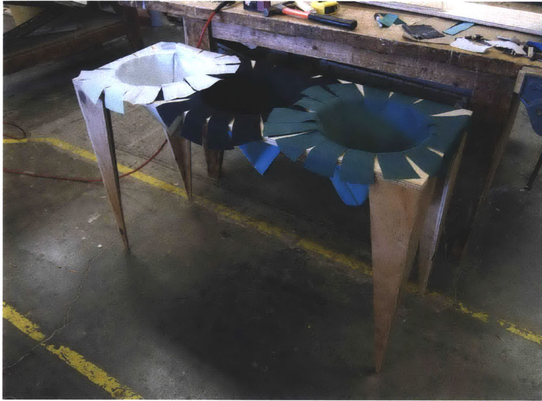
Plate 15 Fabric molds under construction
