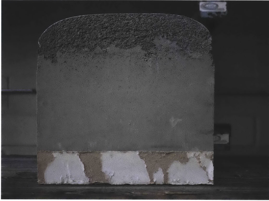
Plate 41 Partially demolded specimen cast in gypsum
