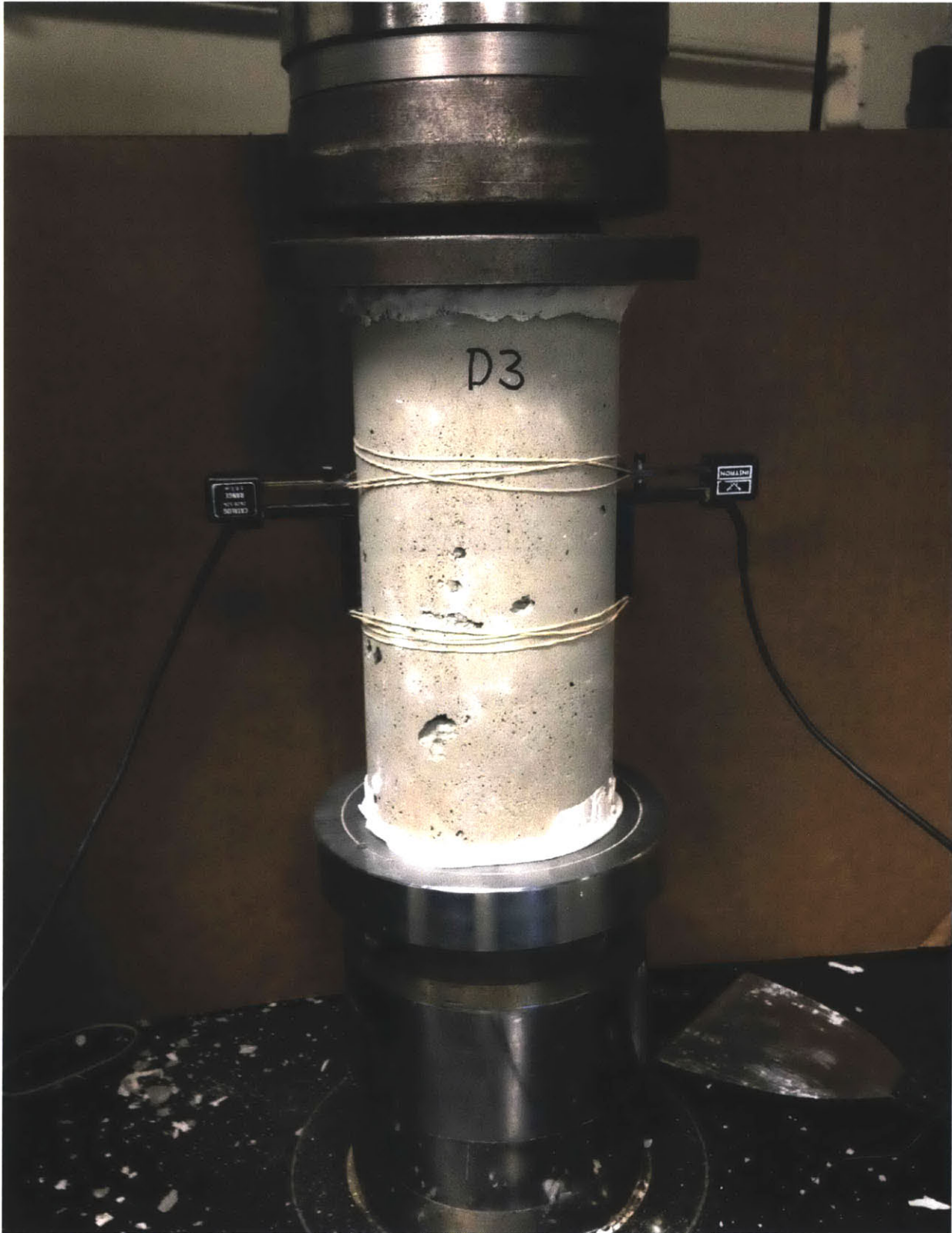
Plate 55 Compression testing setup
