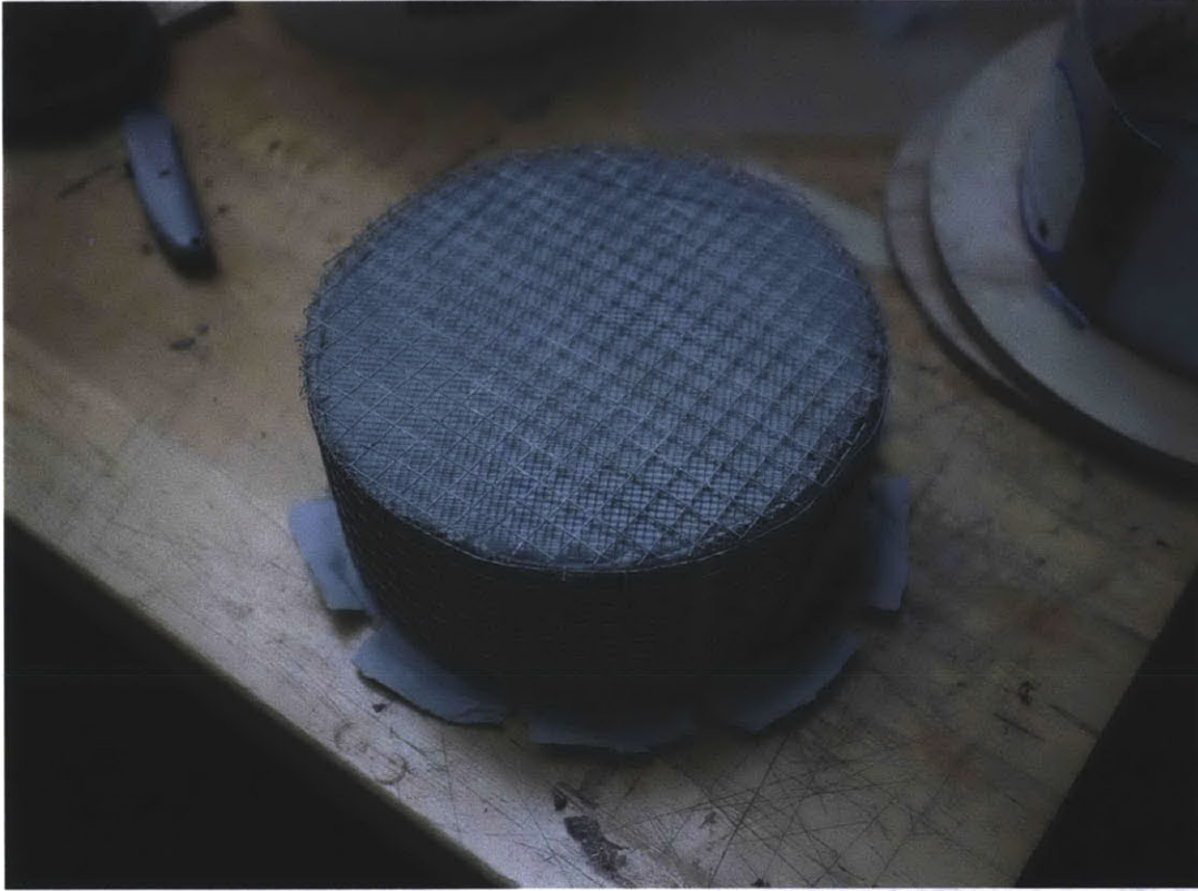
Plate 26 Wire cage and fabric sleeve after demolding
