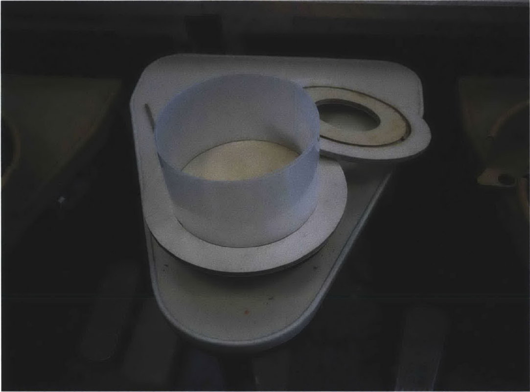
Plate 5 First centrifuge mold
