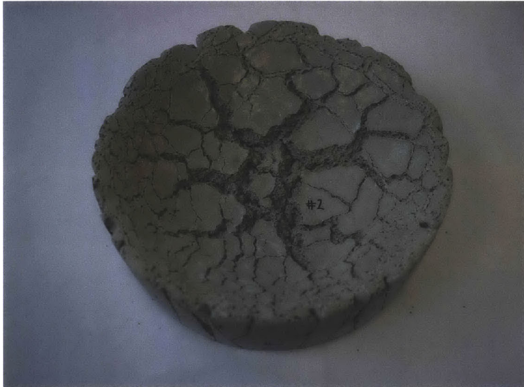
Plate 10 Second centrifuged specimen
