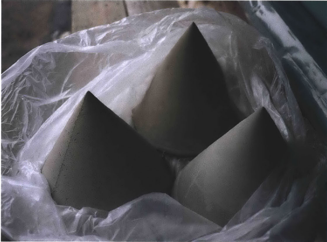
Plate 19 Fabric-formed conical specimens after demolding
