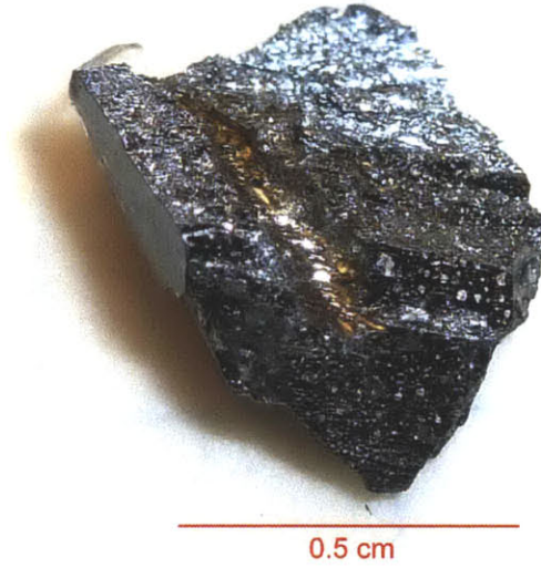
Figure 4-6: Picture of a large \text{In}_4\text{Se}_3 crystal. Because the most easily cleavable, the (1, 0, 0) faces are seen in the plane of the picture.
