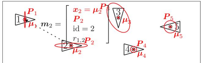
Fig. 1. A set of 5 vehicles performing CN using an EKF. Each vehicle  $i$  maintains the distribution over its state (red) through a mean vector  $\mu_i$  and the associated covariance matrix  $P_i$ . This information, along with the unique ID is broadcasted to other vehicles. Here a broadcast from vehicle 2 is received by vehicle 1.
