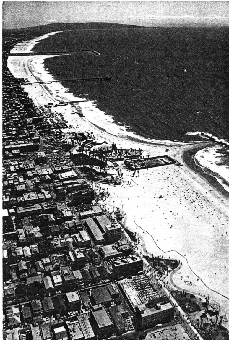
Jetties do not prevent beach erosion. They merely keep sand from drifting on to neighboring sites. Breakwaters are slightly more effective, and are the principle behind constructing new barrier islands.
