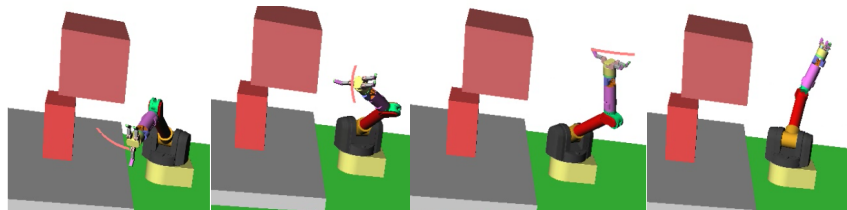
Figure 4-2: Representative test case for the Chekhov Executive. The uppermost portion shows snapshots of the WAM executing the motion plan in the OpenRAVE simulation environment. The middle portion shows the new obstacle that is introduced in the simulation, which prevents the WAM from executing the originally generated plan. The lower portion shows snapshots of the WAM executing a new plan that achieves the original task goal while avoiding the new obstacle.
