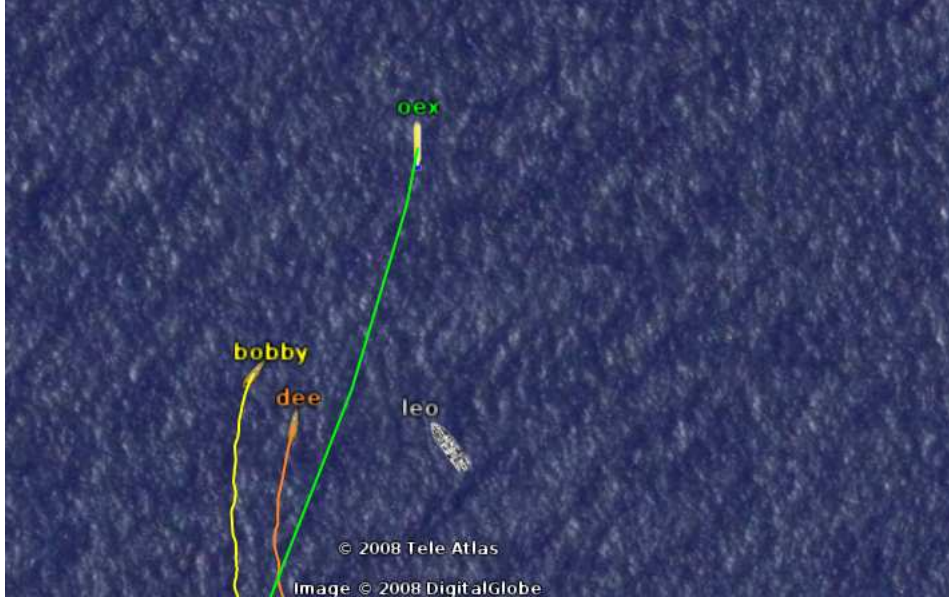
Figure 4: GEOV screenshot showing ASCs Bobby and Dee trailing the OEX AUV to improve networking throughput at the CCLNET08 experiment. Acoustic communications are only robust over short distances with largely vertical propagation, which makes these “mobile gateways” effective, as they can always maintain a relatively short distance to the AUV. The ASCs were commanded to trail at 100 meters behind the AUV at 170^\circ and 190^\circ relative to the AUV’s bow. The ASCs were also running a high priority collision avoidance behavior with the RV Leonardo (“leo”), which accounts for the shift to port from the normative tracking positions.
