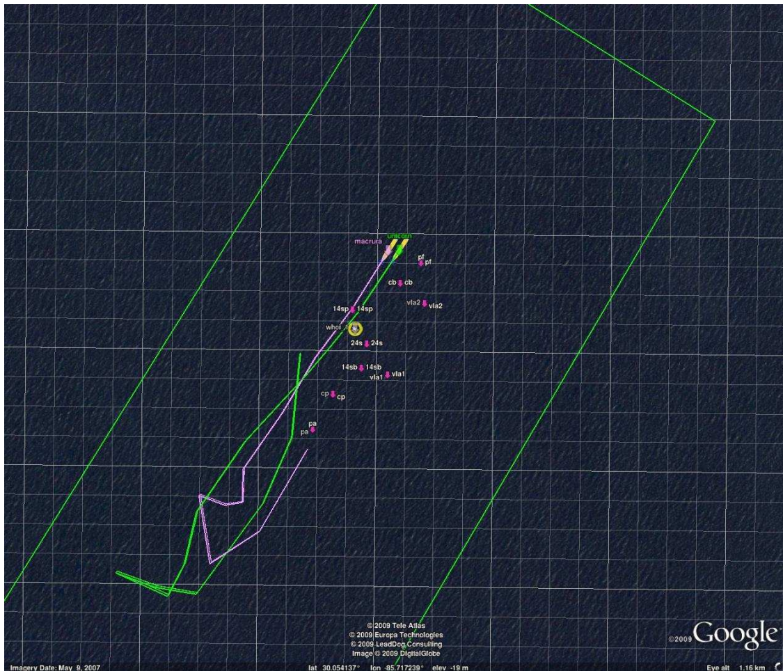
Figure 10: Screenshot of GEOV from the SWAMSI09 experiment. Bluefin 21 AUVs Unicorn and Macrura are performing a synchronized racetrack maneuver for bistatic acoustics (both vehicles have sources and nose arrays). This synchronized behavior was commanded using the LAMSS_DEPLOY DCCL message and is autonomously coordinated using the LAMSS_STATUS message. The history of the vehicles is also provided by the LAMSS_STATUS message. The subsea targets are represented by purple arrows and each grid box is 25 meters square. The solid colored lines indicate the position history of each vehicle, while the name and icon show the current location.
