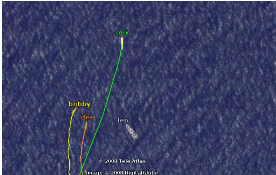
Figure A.4: GEVO screenshot showing ASCs Bobby and Dee trailing the OEX AUV to improve networking throughput at the CCLNET08 experiment. Acoustic communications are only robust over short distances with largely vertical propagation, which makes these “mobile gateways” effective, as they can always maintain a relatively short distance to the AUV. The ASCs were commanded to trail at 100 meters behind the AUV at 170° and 190° relative to the AUV’s bow. The ASCs were also running a high priority collision avoidance behavior with the RV Leonardo (“leo”), which accounts for the shift to port from the normative tracking positions.
