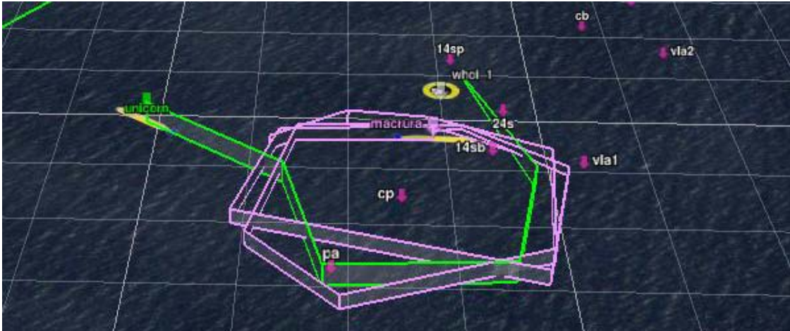
(a) During SWAMSI09, the two AUVs “Macrura” and “Unicorn” perform a synchronous circular pattern with a constant angle of separation. However, due to the sporadic updates from the acoustic modem, it is hard to visualize the performance of the vehicles in executing this maneuver at runtime.
