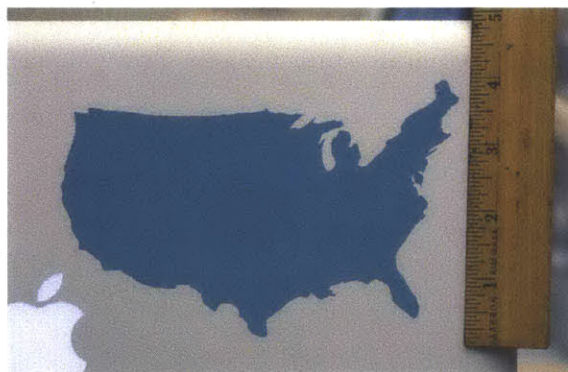
Figure 4-9: Fine details: With a vinyl cutter, the resolution of features is not limited by the width of the bit. Here, we show a 6"-wide sticker with fine details.
