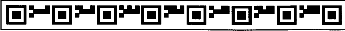
Figure 4-3: Markers: A sequence of markers, with values 1000 to 1006, such as would be printed on a strip of tape. In our current implementation, markers are printed at a size of roughly 0.8'' \times 0.4'' . This is small relative to the area of the material the camera can see at once (roughly 8'' \times 6'' ).
