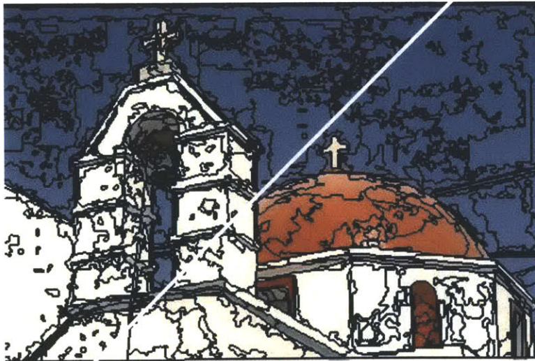
Figure 4-6: Example of the Felzenszwalb algorithm super pixels showing two different parameter settings. The top left favors smaller super pixels while the bottom right favors larger super pixels. Source: Radhakrishna Achanta et al. [1].
