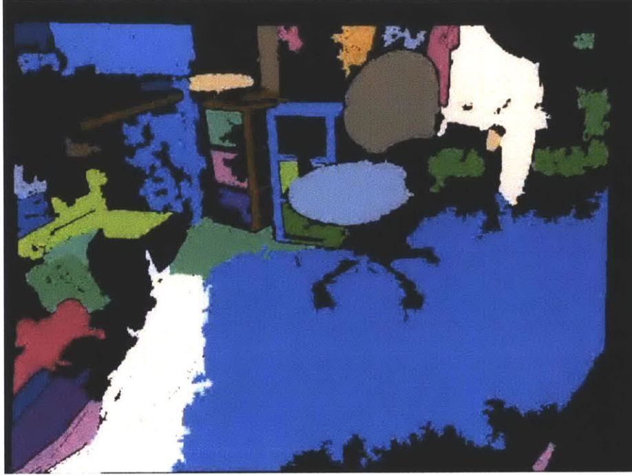
Figure 5-4: Segmentation of RGB-D image from Figure 5-3 colored by unique segment ID.
