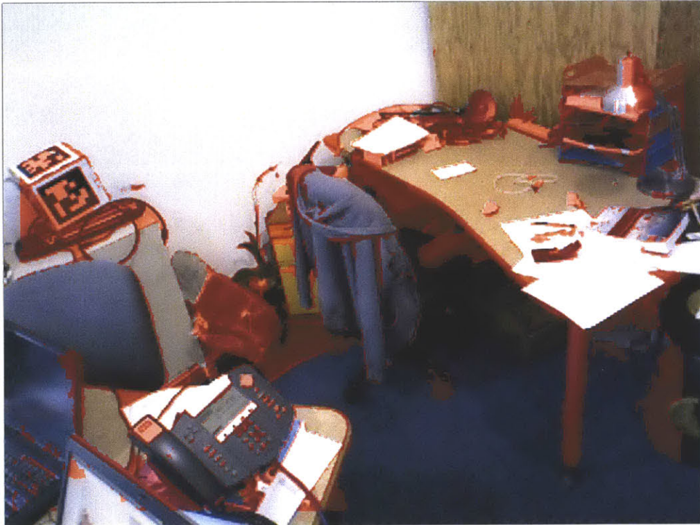
Figure 5-2: An RGB-D image with the unstable (or cluttered) regions highlighted in red. The areas not highlighted in red are deemed stable.
