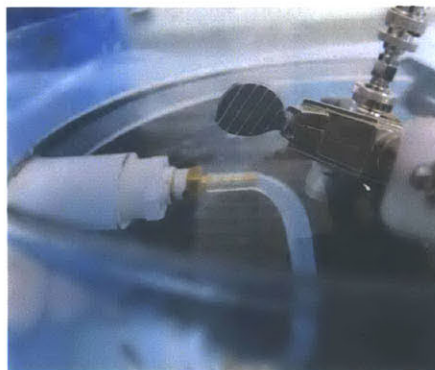
Figure 4-8: Alignment of the ultrasound transducer to the vessel phantom within the experimental flow phantom.
