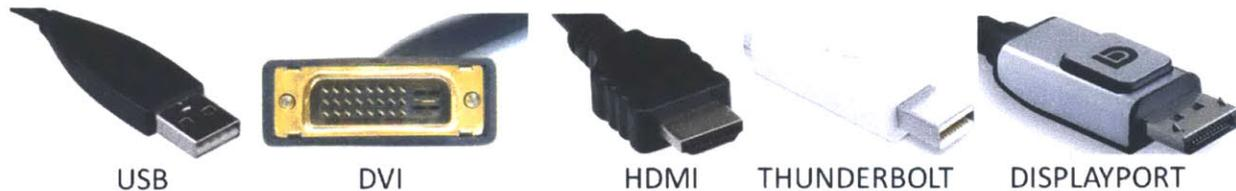
Figure 12. High speed recent PC interface standards
