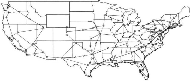
Figure 2-1: The fiber backbone operated by a major U.S. network provider [46]. Node locations are approximate and point-to-point fibers are represented by straight lines.
