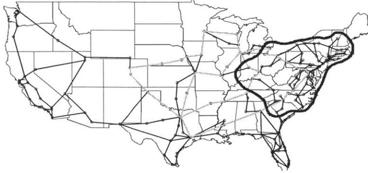
Figure 5-10: Four light grey (teal in online color version) Chicago-Dallas paths are highlighted above for a particular backbone network [46]. The grey closed curve (red closed curve in online color version) surrounding eastern states represents the region of a power blackout. Note the two rightmost paths are not disjoint with respect to this blackout since those pair of data paths both intersect the blackout zone.
