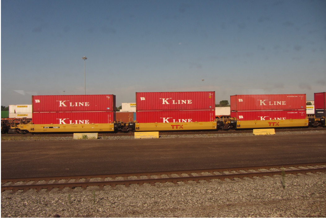
FIGURE 6-1: A 'double-stack' of containers on flat cars in an intermodal transfer yard near Chicago
