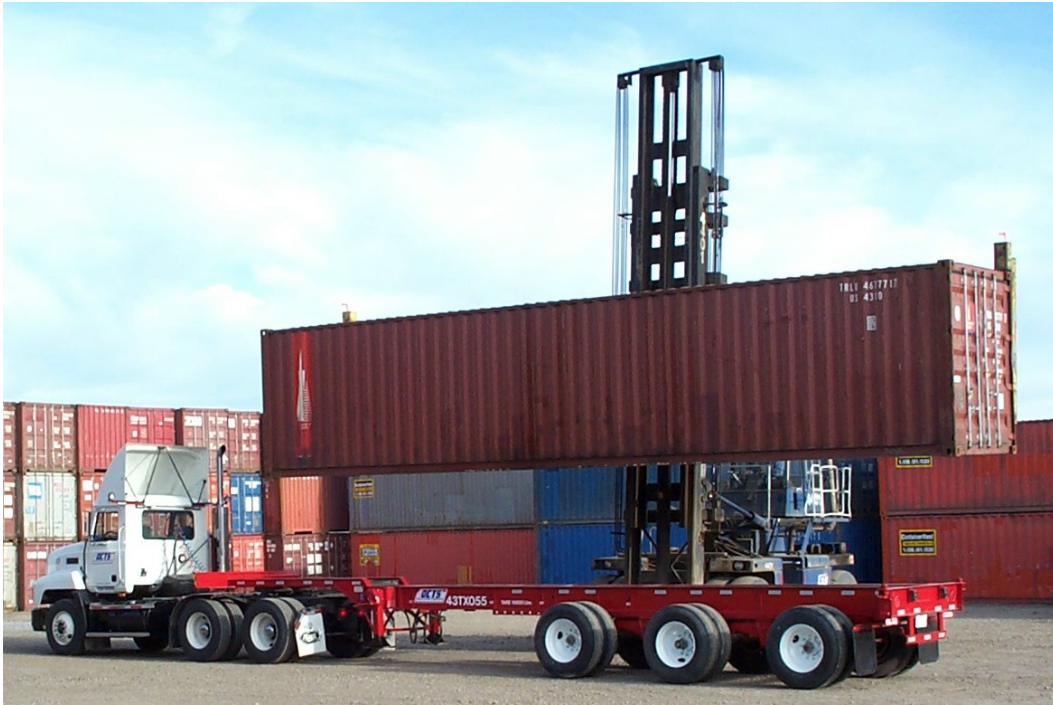
FIGURE 6-2: A container being loaded onto a truck
