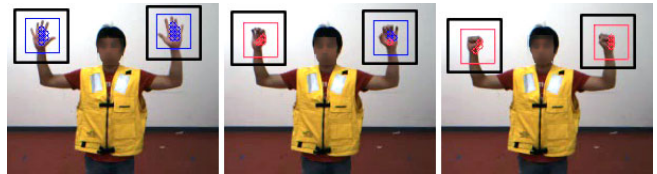
Fig. 5. Search regions around estimated wrist positions (black rectangles). Colored rectangles are clustered results (blue/red: palm open/close), and small circles are individual classification results.
