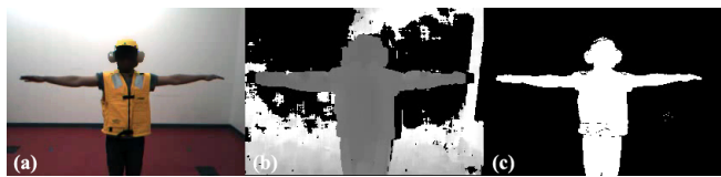
Fig. 1. Example images of (a) input image, (b) depth map, and (c) mask image. The “T-pose” shown in the figures is used for body tracking initialization
