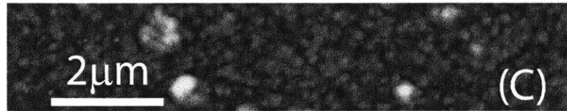
Parylene-C on Au RMS Roughness = 6nm
