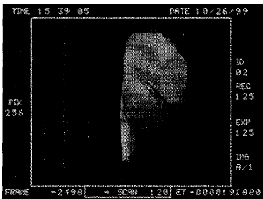
Figure 2-23: Frame obtained from the high speed (1000 fps) imaging of a Ni-Mn-Ga single crystal while the field was ramped up to about 6 kOe.
