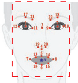
Figure 7: Figure showing the location of the 22 feature points tracked by the Nevenvision tracker. The dashed line highlights the facial region using for evaluating illumination.
