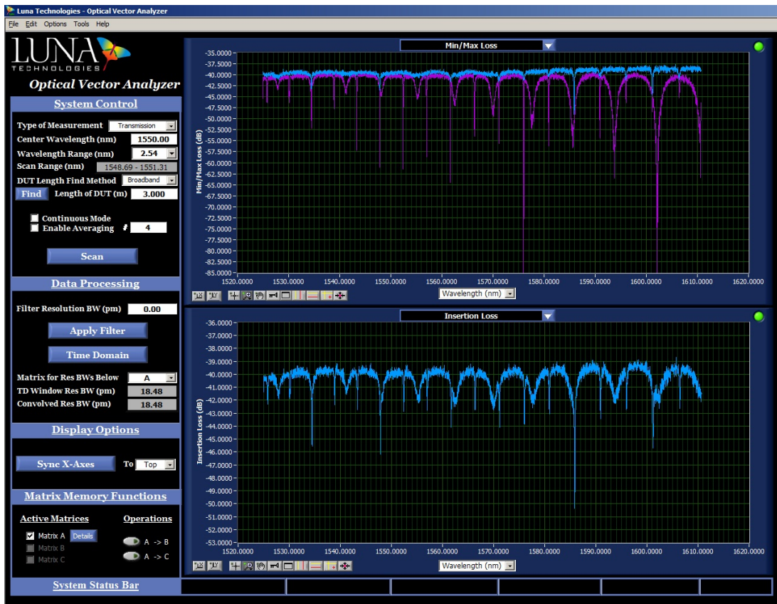
Figure 4-4: Transmission spectrum of a 300 nm \times 220 nm SOI ring (radius: 20 \mu m) with polymer over-cladding measured using the LUNA OVA system.
