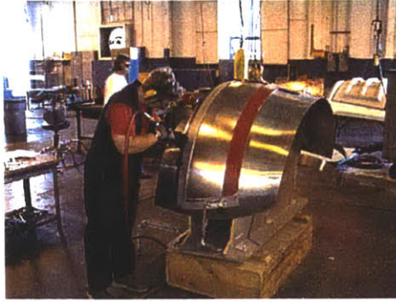
Figure 5.5: Part Being Trimmed.
