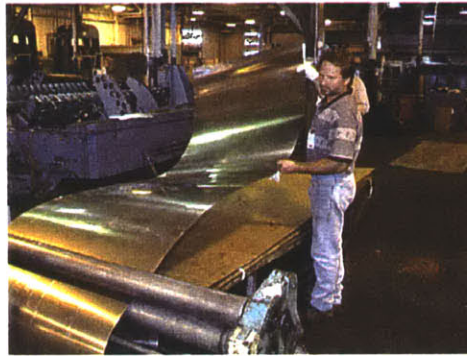
Figure 5.3 Sheet Being Uncoiled.
