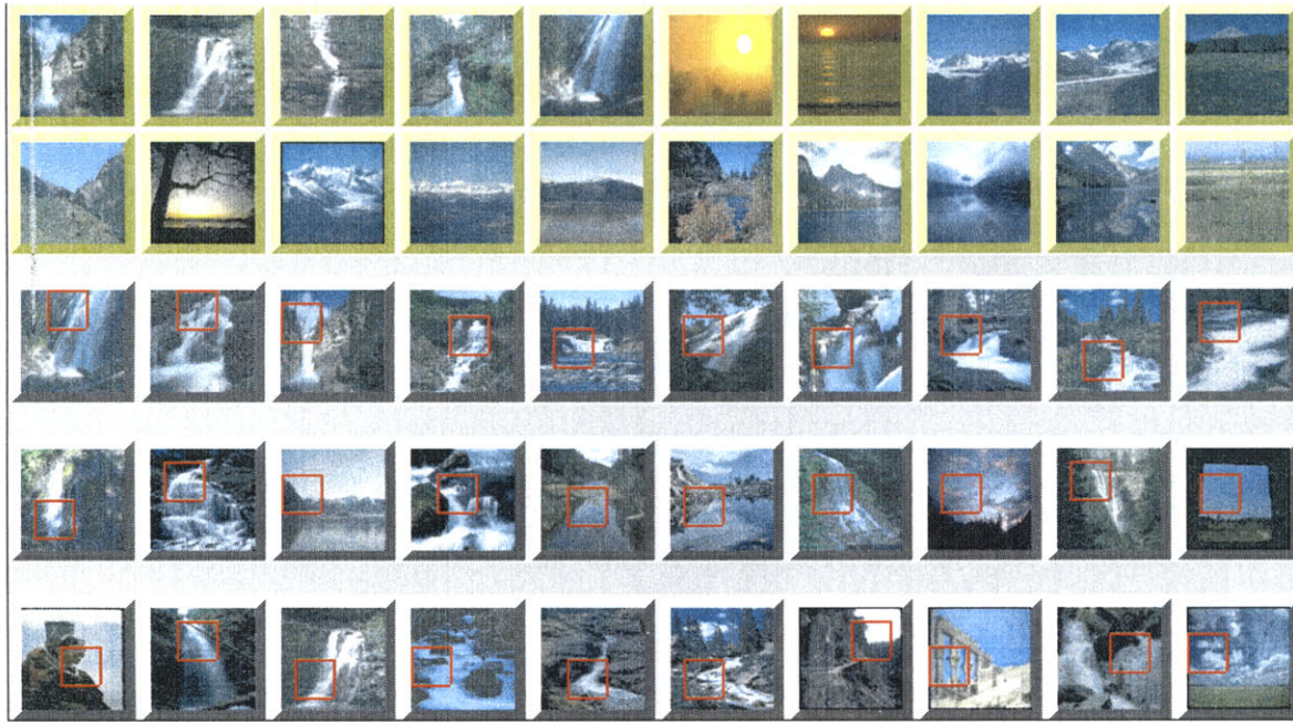
Figure 3-13: Snapshot of the system working. The database contained 2600 images of varied scenes from the COREL library. The figure shows the results for the waterfall class using the single blob with neighbors concept with +10fp . Top row: Initial training set—5 positive and 5 negative examples. Second Row: Additional false positives. Last three rows: Top 30 matches retrieved from the large test set. The red squares indicate where the closest instance to the learned concept is located.
