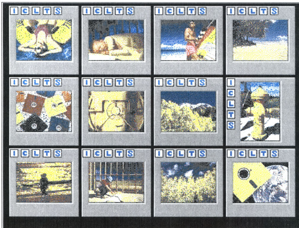
Figure 2-1: This figure shows the set of images retrieved by the QBIC system [Flickner et al. 1995] using global color histogramming. These images are the top few matches that are closest in color composition to the query (first image). The results illustrate that images with very different content can have similar color composition.
