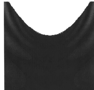
Figure 5.6: Calculated circular and linear polariscope light intensity patterns for the axisymmetric finite point/plane electrode geometry of Figure C.1. The medium is nitrobenzene, the applied voltage is 40 kV, tip-plane distance is 2.5 mm, and point plane electrode radius of curvature is 0.5 mm.
