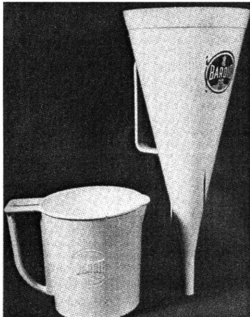
Fig 2.5 Marsh Funnel for Measuring Viscosity (Chilingarian, 1983)
