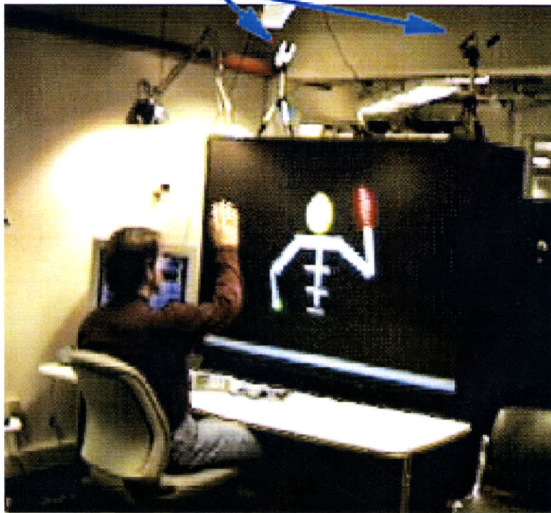
Figure 1-4: The Media Lab's SmartDesk, Tracking hands with Multiple Cameras
