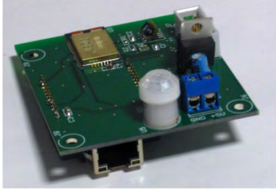
Fig. 4. Room node circuit board.
