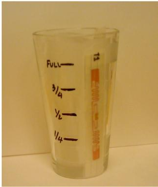
Fig. 3. RFID enabled glass with volume demarcations
