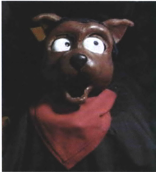
Figure 10-12: Rufus, a simple articulated robot dog head with a camera in its eye. Rufus was the first example of using out pose-blending slime algorithm on a physical robot.
