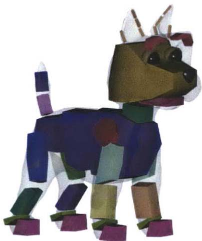
Figure 5-1: The bones (colored solid) which are animated underly the mesh (grey transparent) skin. Each bone rotates with respect to its parent by a 3D rotation, making a hierarchical skeletal model with the pelvis at the root.
