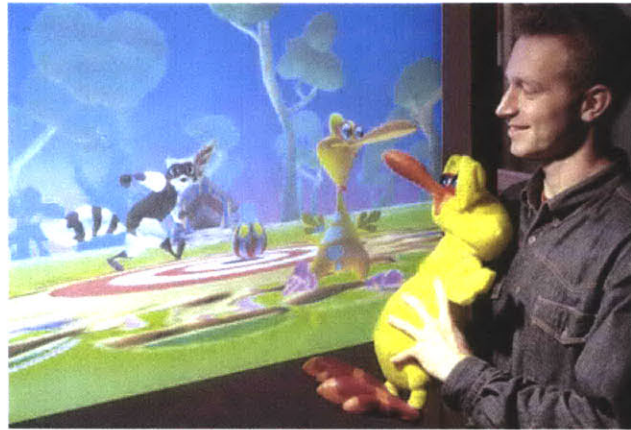
Figure 10-7: The Swamped! project, shown at SIGGRAPH 1998. The interactor directs the chicken character using natural gestures of the plush toy ( sympathetic interface ). The raccoon is autonomous and uses an early slime-based RBF system based on Rose’s Verbs and Adverbs work.
