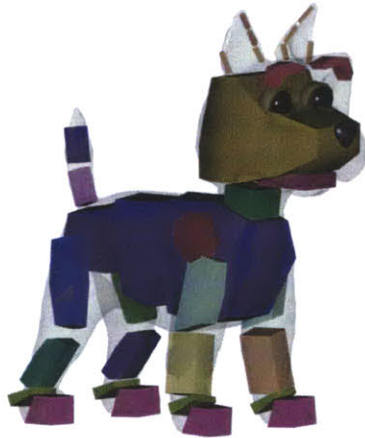
Figure 1-2: The bones (colored solid) which are animated underly the mesh (grey transparent) skin. Each bone rotates with respect to its parent by a 3D rotation, making a hierarchical skeletal model with the pelvis at the root.
