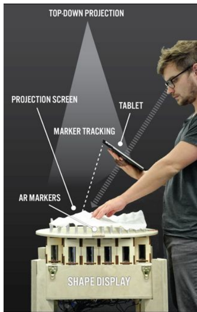
Figure 5: Multi-user setup, using handheld tablets to augment the shape display through video see-through AR.
