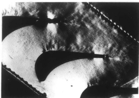
Figure 4.24b Reference Blade 1 Schlieren photos g/c = 0.81
