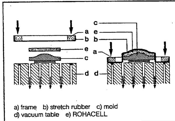
Fig. 45: Forming ROHACELL with stretch rubber
