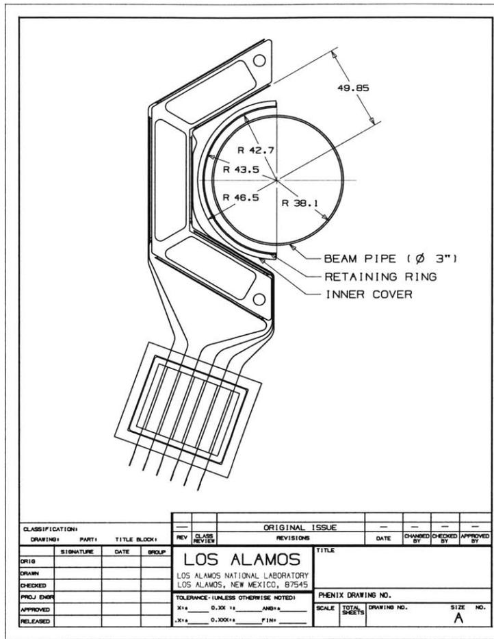
**Figure 4-2: Clearances around the inner Rohacell cover**
