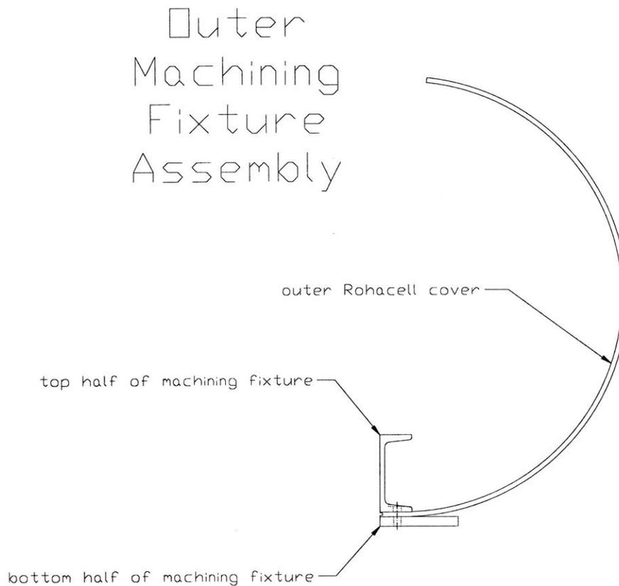
**Figure 5-3c: The outer cover machining fixture assembly**
