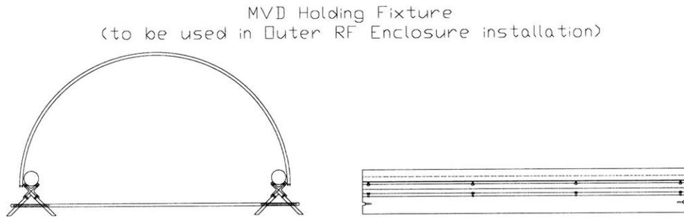
**Figure 5-6a: Conceptual assembly drawing of MVD holding fixture**
