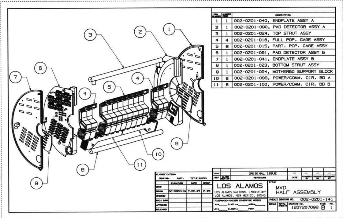
Figure 1: Exploded isometric view of the assembled RF Enclosure
