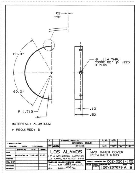
Figure 5-4: The inner enclosure retaining ring
