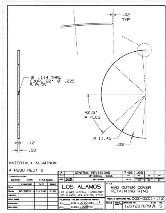
Figure 5-5: The outer enclosure retaining ring
