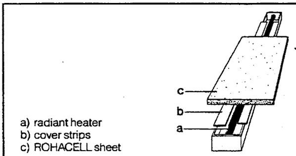
Fig. 39: Line bending of thin ROHACELL sheets
