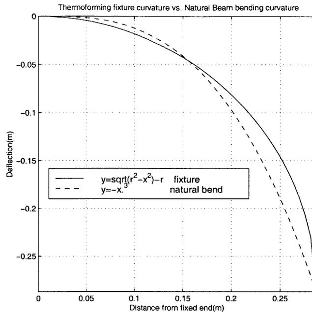
**Figure 5-1: Thermoforming fixture vs. Rohacell bending curvatures**
