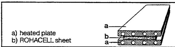
Fig. 38: Heating between plates
