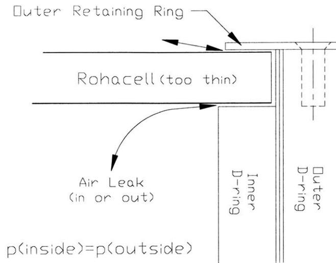
**Figure 3-2: Outer enclosure air leak possible flow path**
