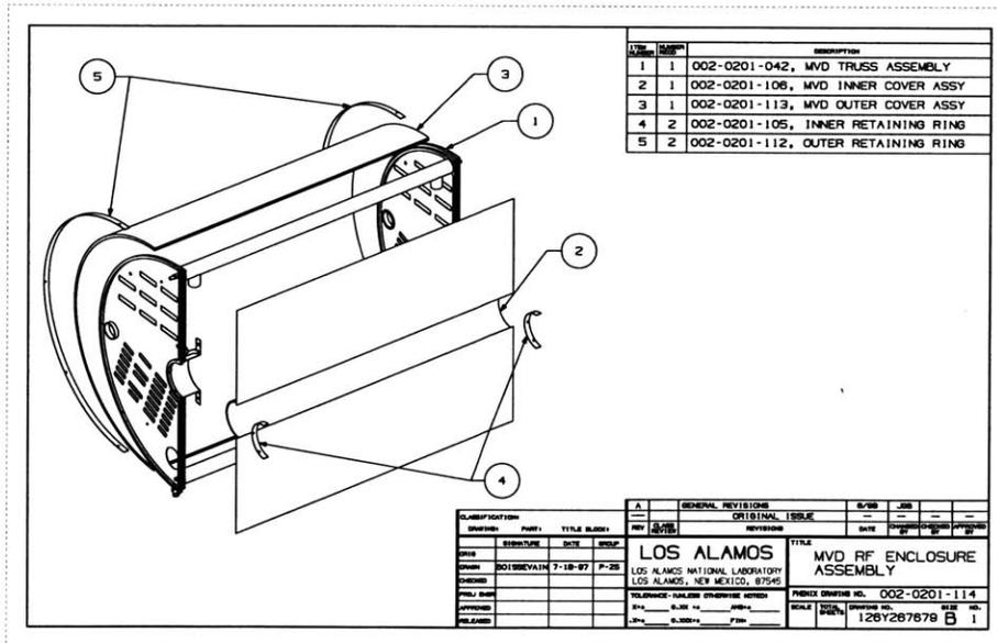
**Figure 1: The MVD's Radio Frequency Enclosure**
