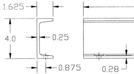
**Figure 5-3b: Enlarged view of top plate (C-beam)**
