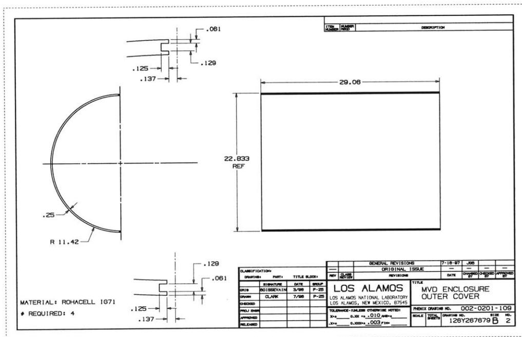
**Figure 2: The Outer Enclosure's Rohacell Cover**
