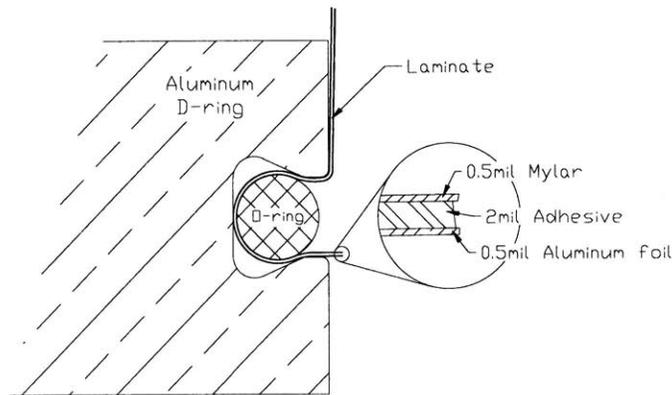
**Figure 3-1: Detail of O-ring groove and enclosure laminate**
