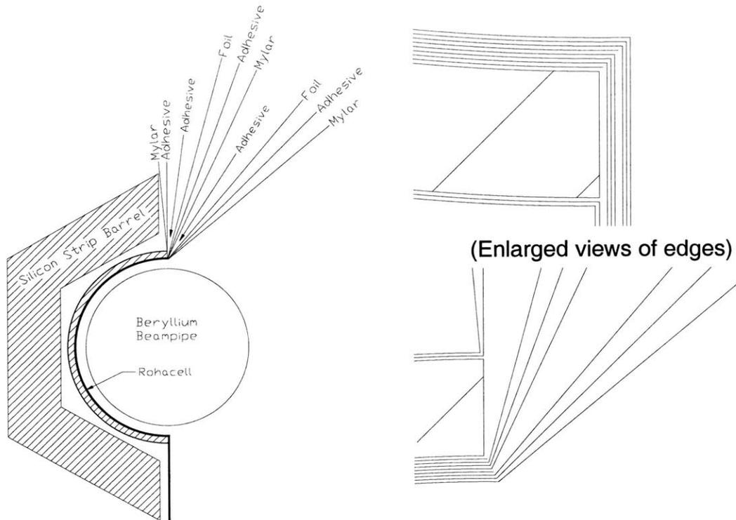
**Figure 4-3: Layers of the inner RF enclosure**
