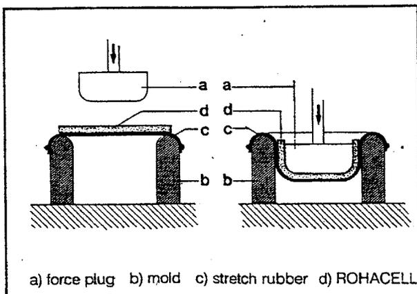
Fig. 43: Forming a shell with stretch rubber
