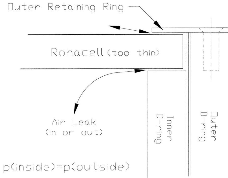
**Figure 5-7: Model of possible air leak path**
