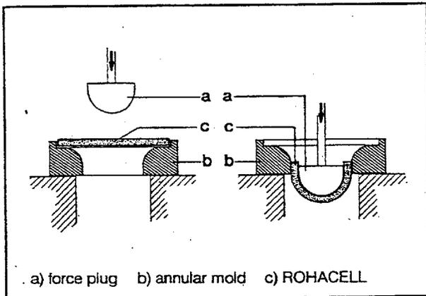
Fig. 42: Forming of a hemisphere from ROHACELL
