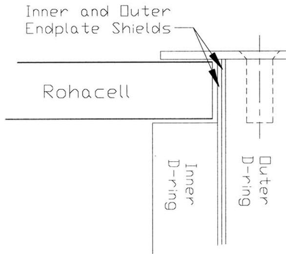
**Figure 3-3: Cross-section detail of D-rings and endplates**
