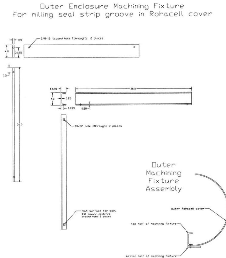
**Figure 5-3a: Base plate, top plate (C-beam), and assembly,**
