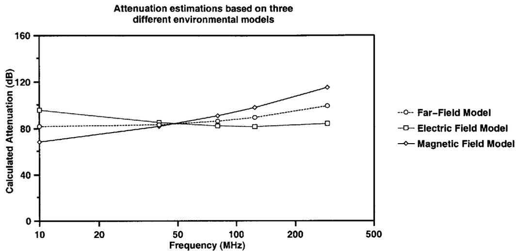
**Figure 2-1: RF shield attenuation estimations using different source models**
