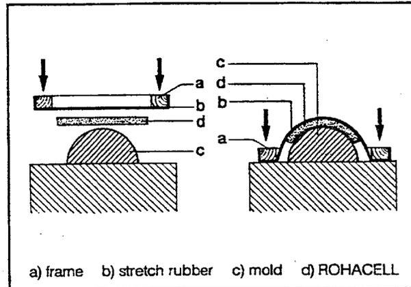
Fig. 44: Forming ROHACELL with stretch rubber
