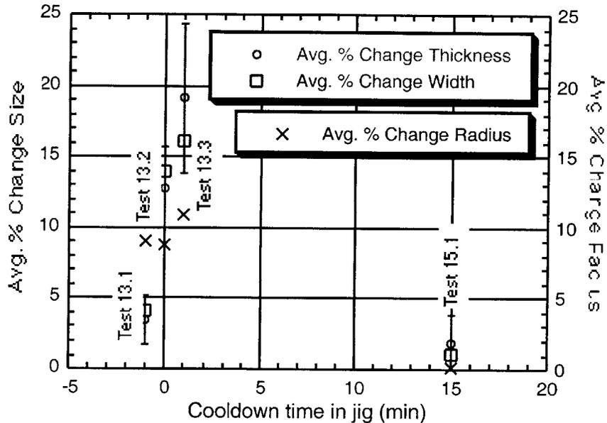
(Test 13.1 did not have a negative cool down time, and Test 13.3 did not have a cool down time of one minute. Rather, they both were allowed to cool down for zero minutes, but are spread apart to distinguish their separate values.)
