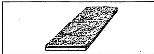
Fig. 41: ROHACELL sheet covered on one side only
