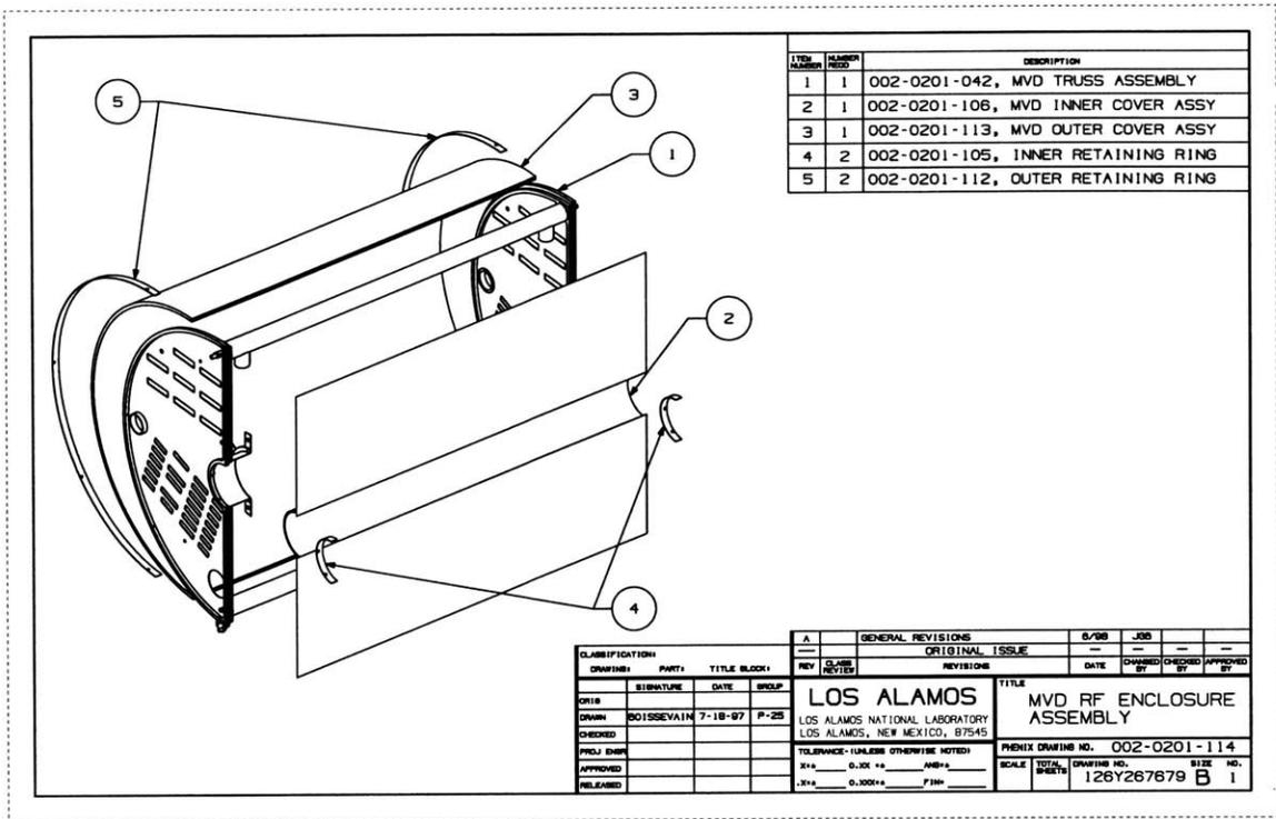
**Figure 1-4: Exploded view of the MVD's RF Enclosure**
