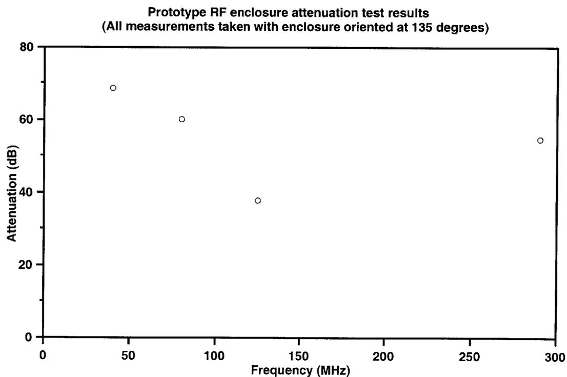
**Figure 6-3: Variation of attenuation with transmitted frequency**
