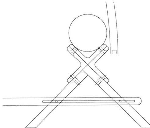
**Figure 5-6b: Enlarged end-view with Rohacell and strut in place**
