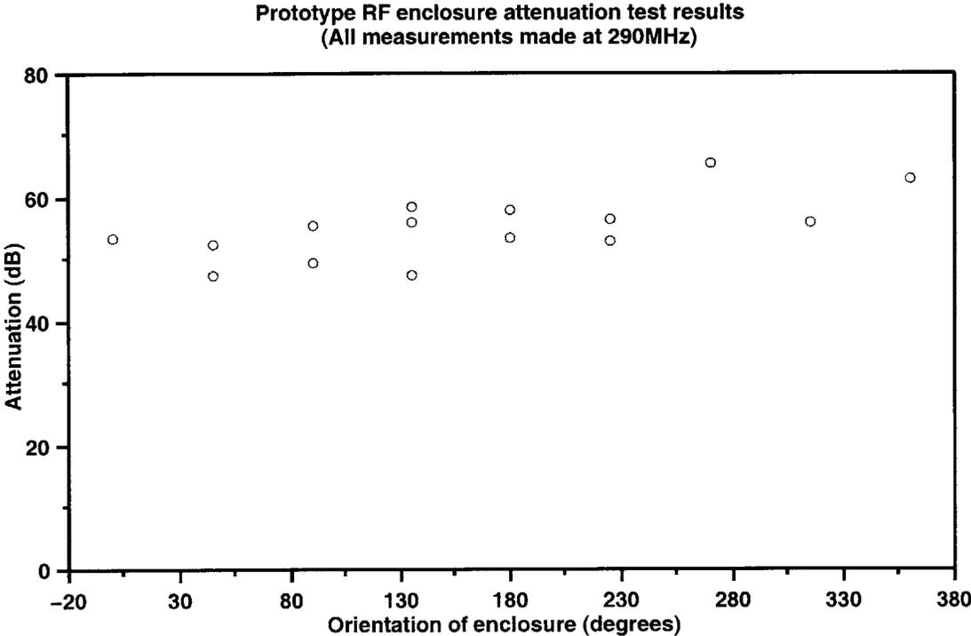
**Figure 6-2: Variation of attenuation with enclosure orientation**
