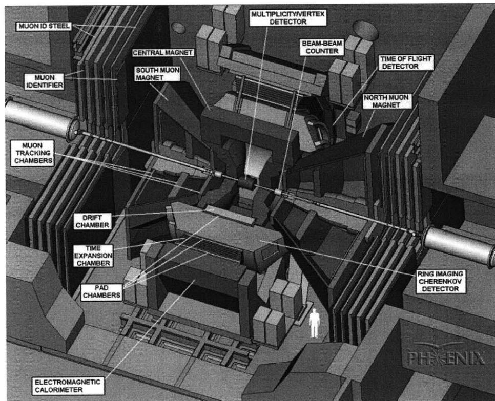
**Figure 1-2: The PHENIX experiment's detector layout**
