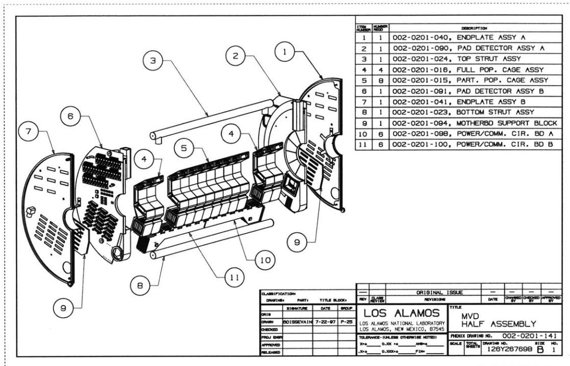
**Figure 1-3: Exploded assembly drawing of one half of the MVD**
