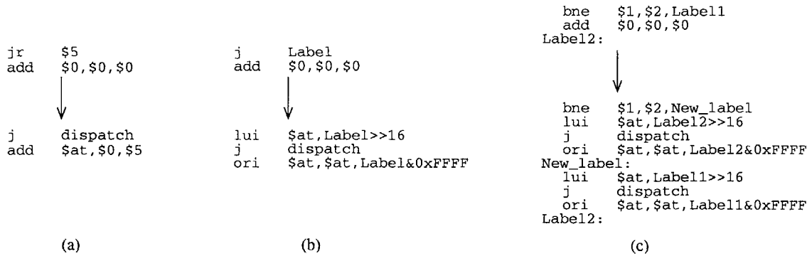
Figure 3-1: Example replacements of (a) a jr instruction, (b) a j instruction and (c) a conditional branch instruction.
