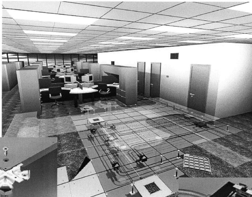
Figure 14: Typical interior with raised floor systems, partitions [13]
