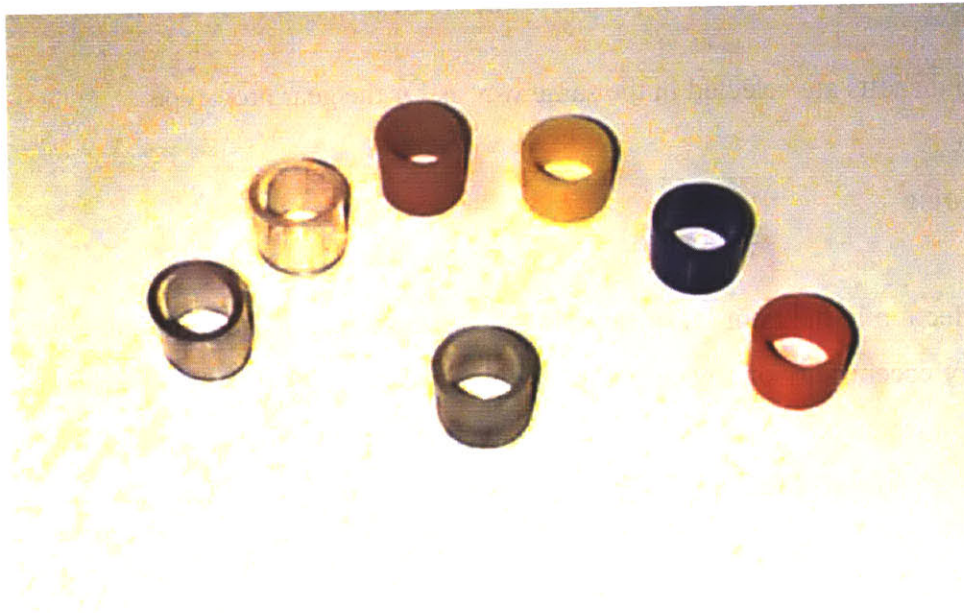
Figure 4.19 Flexible Tube Materials (Left to Right: PVC, ether-based polyurethane, natural rubber, ML6 Plastic 30, 40, and 50 durometer. Center: ester-based polyurethane)
