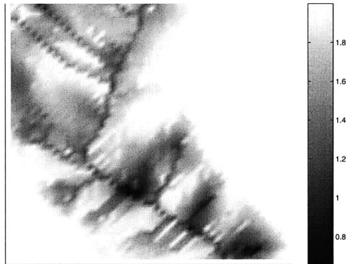
Figure D-1: Map of water table depth for 2-km 2 square subsection of Bear, CA.
