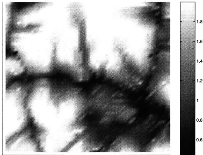
Figure D-10: Map of water table depth for 2-km 2 square subsection of Yreka, CA.
