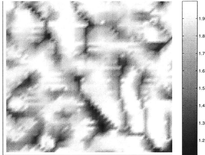
Figure D-2: Map of water table depth for 2-km 2 square subsection of Brushy, AL.
