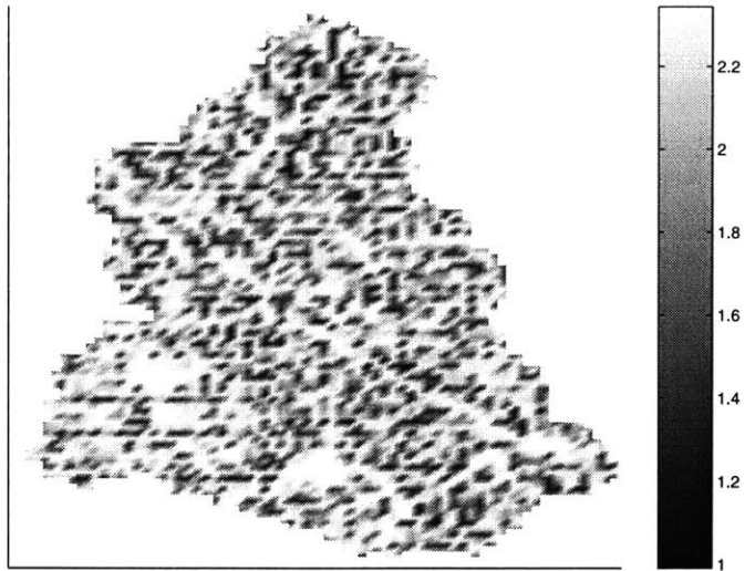
Figure 5-8: Diffused distribution of soil depths calculated from the Dietrich et al. model, Midland, VA.
