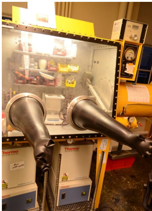
Figure 1.4: (A) Picture of glovebox and attached furnace used for testing. (B) Picture of a batch of four cells labeled after base component cleaning. It is important to note that these four cells, with mild steel PCC, were not used for this study and are simply to demonstrate labeling procedure.
