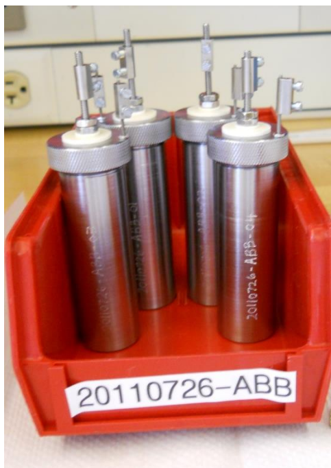
Figure 1.4: (A) Picture of glovebox and attached furnace used for testing. (B) Picture of a batch of four cells labeled after base component cleaning. It is important to note that these four cells, with mild steel PCC, were not used for this study and are simply to demonstrate labeling procedure.
