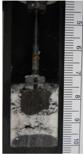
Figure 2.7: Picture of a 20121219-ABB-04 cell post-mortem, scale is in units of centimeters. This cell was manually stopped while in the complete charged state.
