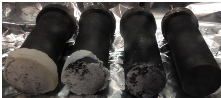
Figure 4.9: Depicts a batch of four 20121202 Li-Mg/LiCl-KCl/Sb-Pb cells ordered 1-4 from left to right. Cells 01 and 02 cycled longer and observed regular resistance spikes, cell 03 did not cycle as long, and cell 04 suffered from a connection failure not cycling at all.
