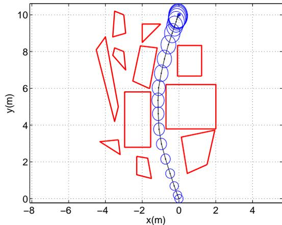
**Fig. 8.** Example solution with hard map and  $\Delta = 0.001$ . The goal is shown as the small blue square at  $(0, 10)$ . The dots show the mean of the planned UAV position at each time step, and the ellipses give the 99% certainty region for the position.
