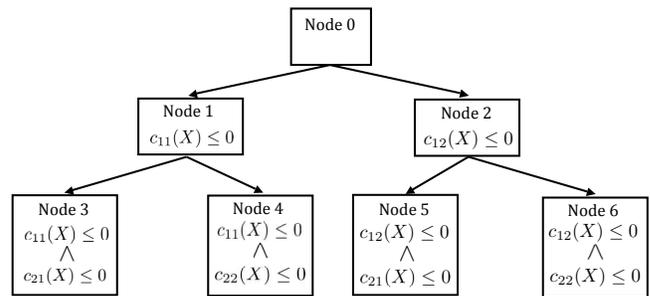
**Fig. 15.** Example search tree for general disjunctive convex program. In this case  $n_{dis} = n_{cl} = 2$ . Shown in the boxes are the inequality constraints applied at that node. Nodes are expanded to their children by branching on disjunctions and adding constraints to those imposed at the parent node. The equality constraints (not shown) are applied at all nodes.
