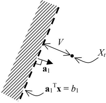
**Fig. 4.** Linear constraint and vehicle position  $X_t$ .  $V$  is the distance between the constraint and the vehicle, defined as positive for values of  $X_t$  for which the constraint is satisfied, and negative for value of  $X_t$  for which the constraint is violated. The vector  $\mathbf{a}_1$  is the unit normal in the direction of positive  $V$ .
