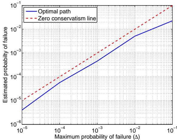
**Fig. 12.** Estimated probability of failure against maximum allowable probability of failure  $\Delta$ . For comparison we show the line with unity gradient that corresponds to zero conservatism. The chance constrained plan is conservative by a factor of approximately 2.
