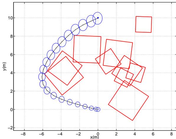
**Fig. 13.** Typical randomly generated map and path generated by customized solution method. The dots show the mean of the planned UAV position at each time step, and the ellipses give the 99% certainty region for the position.
