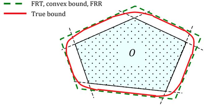
**Fig. 6.** Obstacle from Figure 2 and illustration of bounds. The lines show the feasible regions for a given value of  $\Delta$  for the various bounds introduced in this paper. Note that since we have a single obstacle and time step, the convex bound, FRT and FRR are identical.
