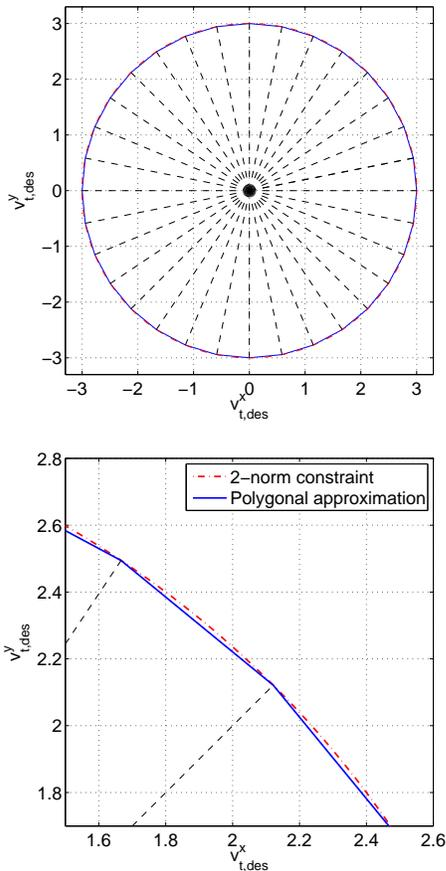
**Fig. 7.** Approximation of 2-norm constraint as 32-sided polygon. This approximation is used both in bounding the velocity of the UAV to 3m/s (as shown here) and in computing the cost of the planned path, which is proportional to the 2-norm of velocity.
