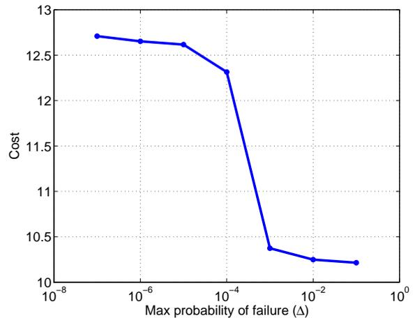
**Fig. 10.** Cost of returned solution against  $\Delta$ . As the maximum allowable probability of failure specified by the operator increases, the cost decreases monotonically. The sharp drop corresponds to finding the path through the narrow corridor.
