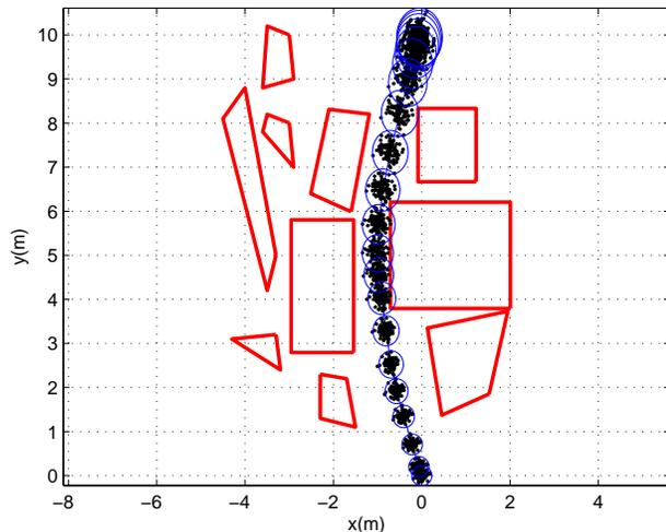
**Fig. 14.** Typical solution generated by particle control approach for the hard map, with  $\Delta = 0.01$ . The black dots show the 100 particles used in the plan. At most one particle can violate the constraints. The blue ellipses show the 99% certainty region for the position.
