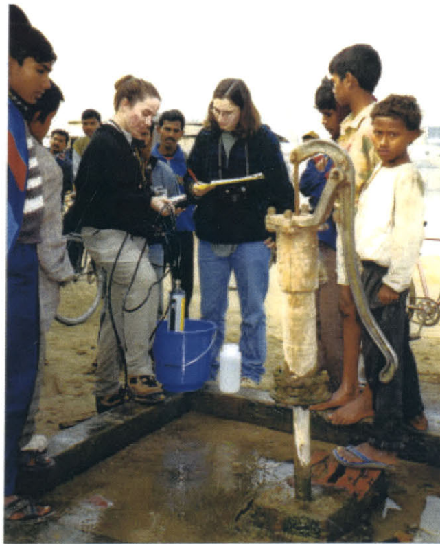
Figure 4.3: Typical tube well in Nepal
