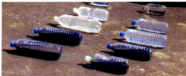
Figure 7-1: Bottles undergoing solar disinfection
