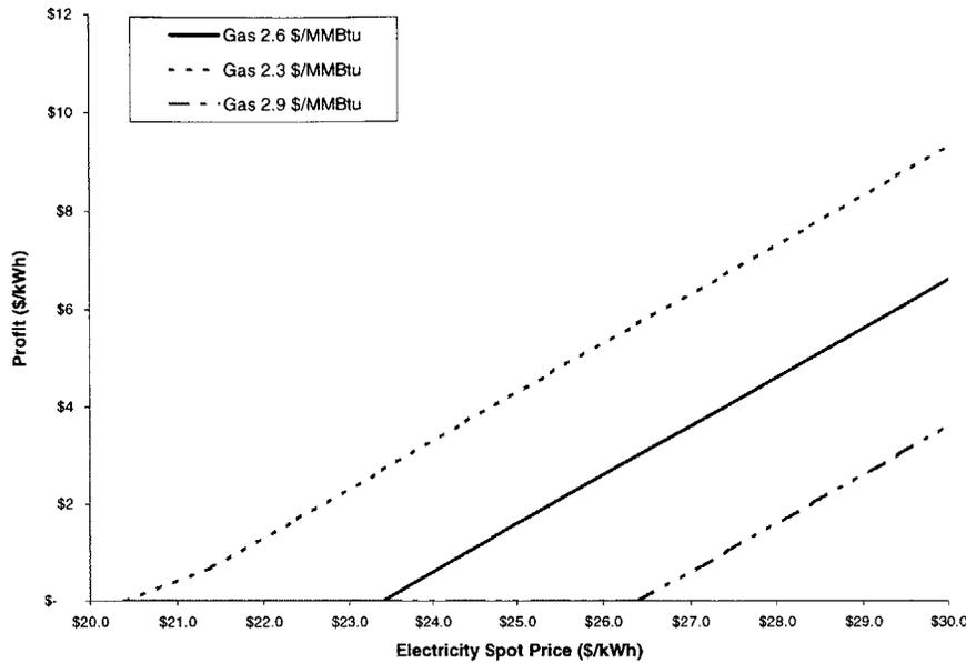
Figure 6.1: Profit curves for different electricity and gas prices.
