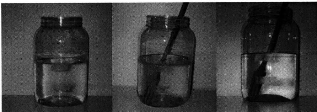
FIGURE 5-7: MANUAL COAGULATION AND SETTLING EXPERIMENT. (A) RAW WATER; (B) AT START OF SETTLING TIME; (C) AFTER 30 MINUTES OF SETTLING.
