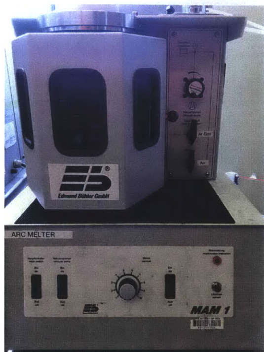
Figure D-2: Arcmelter used to prepare the reference electrodes.
