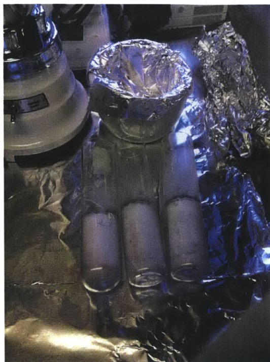
Figure D-1: Pre-melted salts inside quartz crucibles before
