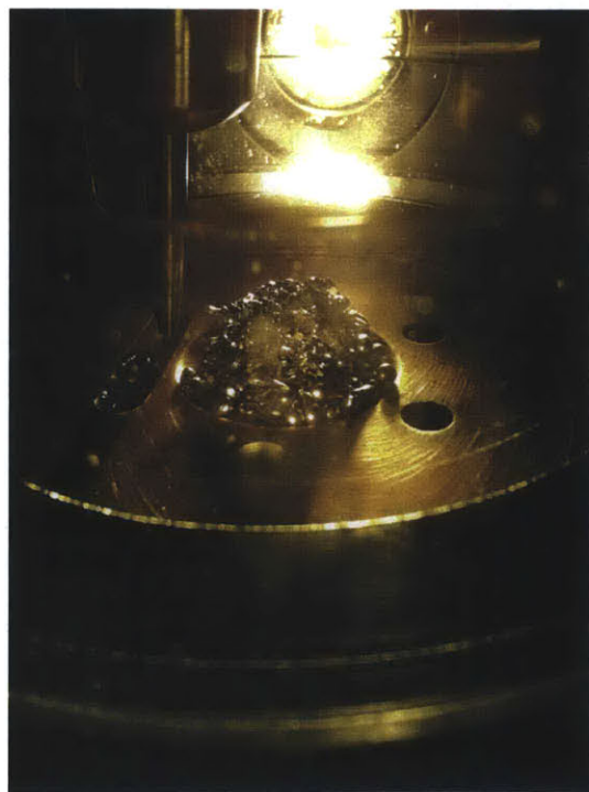
Figure D-3: Calcium and bismuth metals inside arc-melter.
