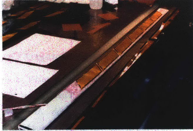
Figure 1-2: AFC being inserted at active blade assembly
