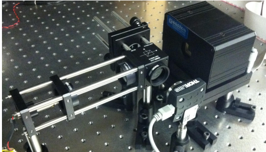
(a) CubeSat-scale MEMS DM Michelson interferometer
